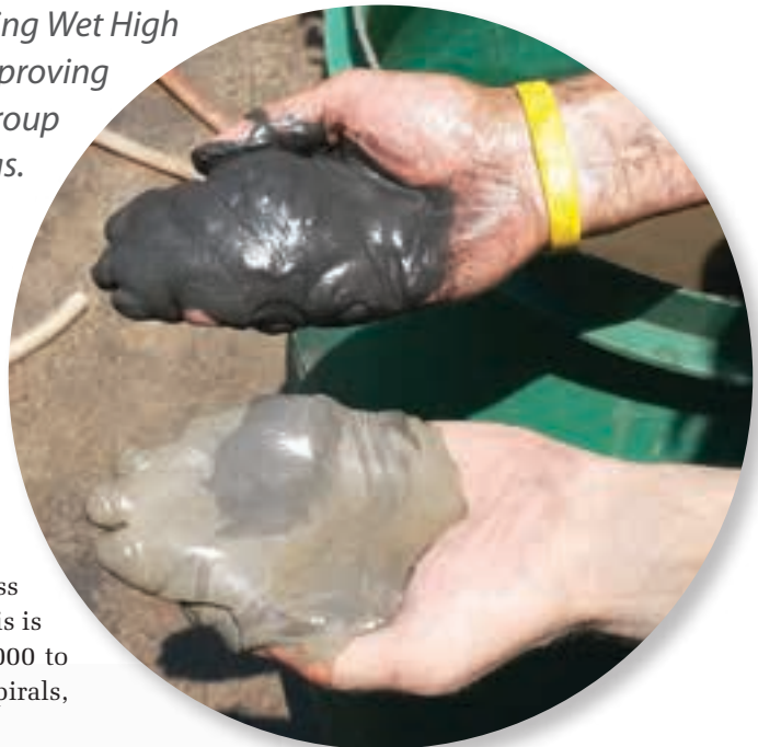
Above: Slimes dam ultra fine chrome separated from PGM containing silica with a Longi-Multotec vertical ring WHIMS machine.
