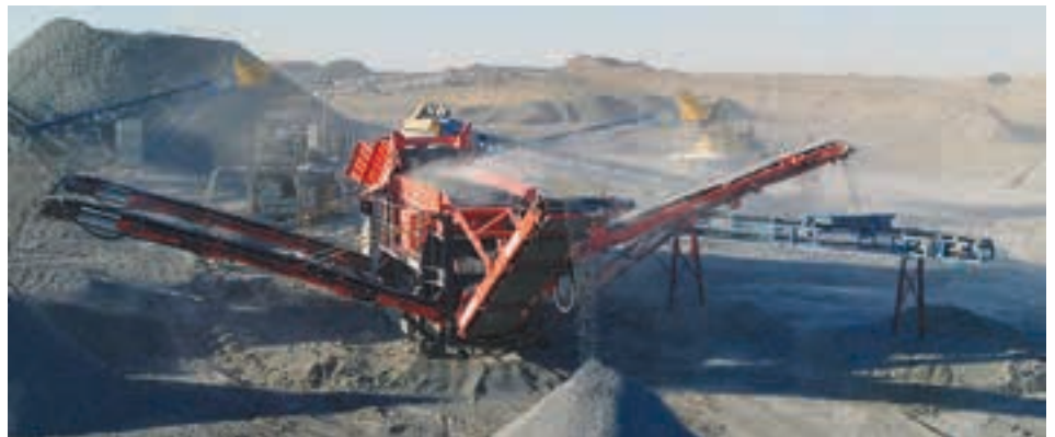
The track-mounted, mobile triple-shaft, triple-deck horizontal screen is designed to produce as many as four products simultaneously.
