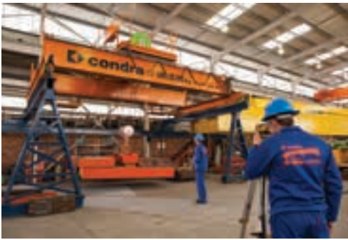
Load testing on one of the two 25-ton headgear cranes manufactured by Condra for Mopani Copper Mines' Synclinorium shaft.
