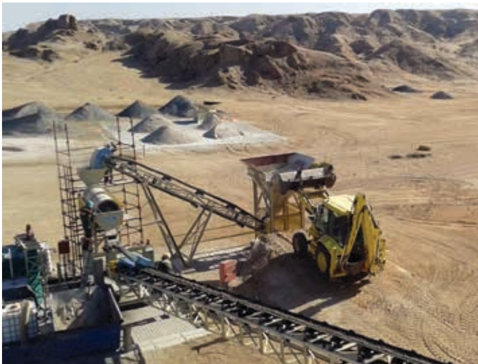
The ore was fed into the agglomeration drum via a conveyor at a controlled feed rate, and agglomerated through adding sulphuric acid, a polymer binder and water to produce agglomerated ore with properties as per DFS specifications. Agglomerate samples were taken from the stacking conveyor on an hourly basis and analysed for moisture content (photo: Bannerman).
