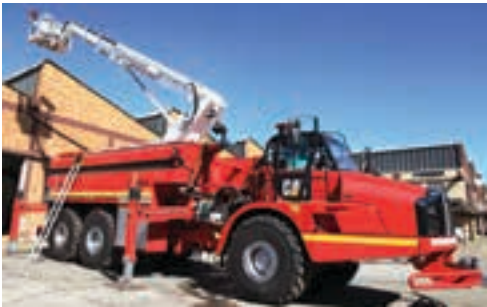
During a fire, the main tank has the capability of deploying 2 900 litres per minute from a height up to 28 m and an estimated range of close to 45 m.
