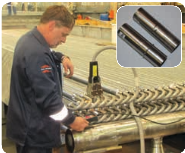
Above: For tube-to-tubesheet welding, Kelvion Thermal Solutions has developed a modified orbital welding technique using copper weld retainers that enables single-pass welding without any overlap into the tube bore. Left: Kelvion Thermal Solutions has developed a way of tube-to-tube welding on serpentine heat exchangers. The method uses filler-metal inserts (inset) to enable an orbital system to be used to complete each weld in a single pass without under filling the joint.
