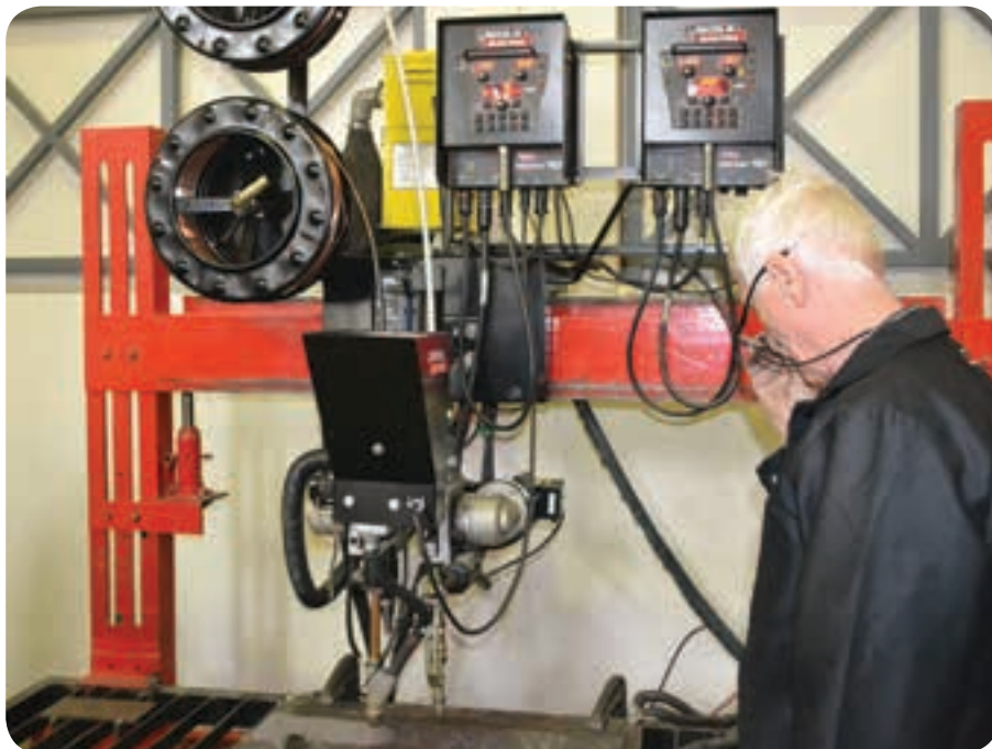
Josef Henning demonstrates submerged-arc welding using a Power Wave 1000 SD in dc constant current mode.
