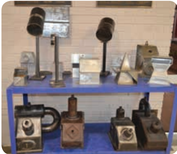
A collection of past welding projects completed by contestants in SAIW's welding challenges. As well as plate and pipe welds in steel, stainless steel and aluminium, contestants are also required to assemble and weld projects from given blueprints, the most onerous being the carbon steel pressure vessel project (bottom shelf).
