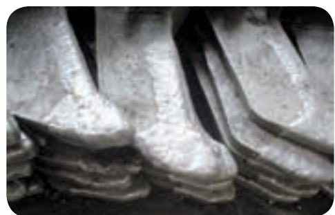
Dedicated UTP sugar segment SMAW and FCAW products for repairing hammers, knives and mill rolls for cane crushing and shredding are currently "outperforming anything else on the market".
