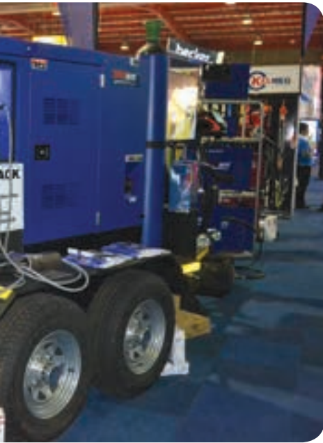
Two independent welding power sources are incorporated allowing two welders to operate simultaneously off the same welding generator.
