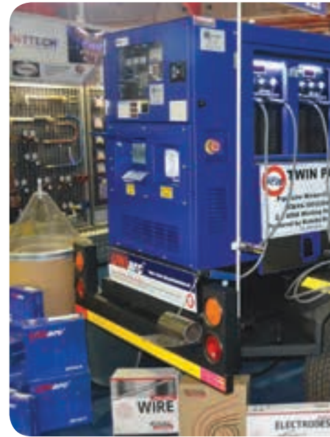
The centre piece of Renttech SA's stand at Electra Mining 2016, the new Uniarc Twinpro twin pack welder/generator powered by a four-cylinder Kubota engine running at 1 500 rpm for reduced maintenance.
