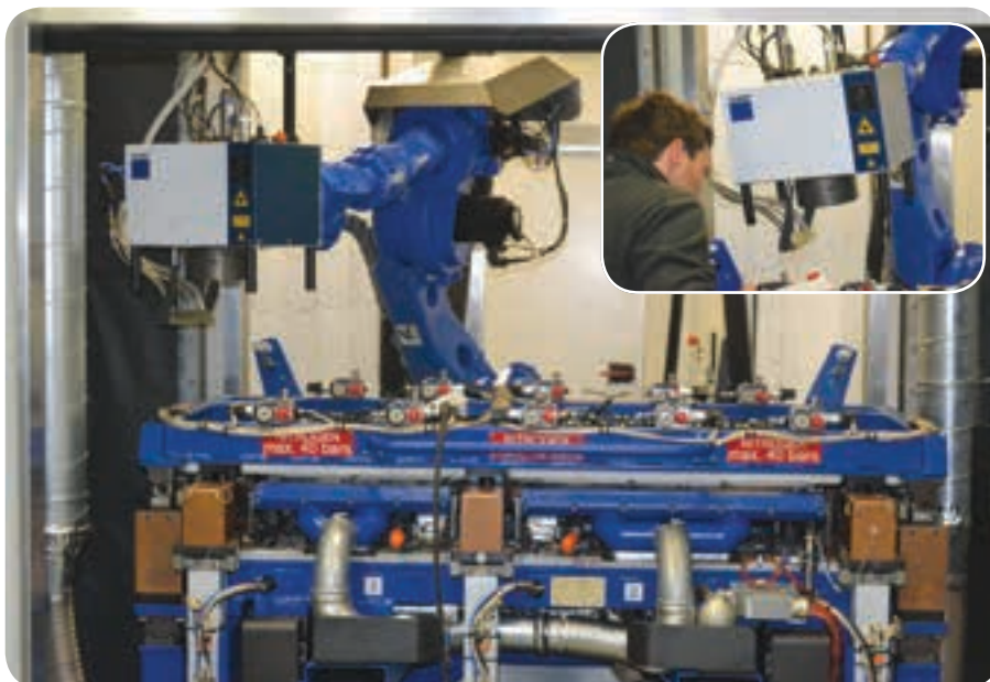
A 6.0 kW Trumpf TruDisk 6002, diode-pumped, solid-state disk laser is used to generate the laser beam, which is fibre-guided to a laser head (inset) with programmable focusing optics (PFOs) on the end of the Yaskawa robot.
