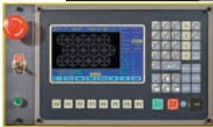
Above: A mechanised plasma torch and a Crossbow CNC cutting system convert a cost-effective Cutmaster plasma cutter into a simple, compact, portable and very economical CNC cutting system. Left: An HMI screen and CNC control panel enable simple profiles to be programmed directly into the system and a library of basic shapes is available to further simplify this process.
