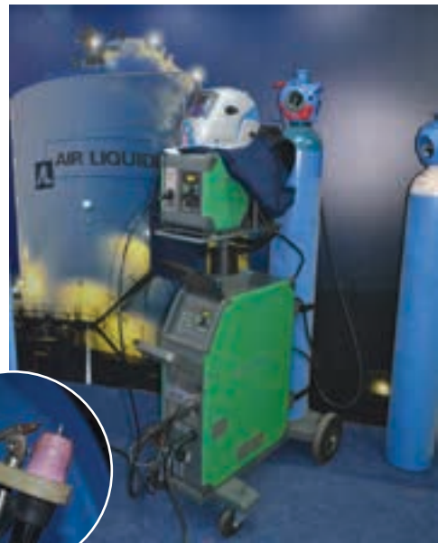
Migatronic's Pi 320, 400 and 500 for TIG welding are available with two different control panels, TIG HP and TIG AC/DC, both of which feature IGC. Inset: A cold wire feed system for TIG welding using the Migatronic Pi.
