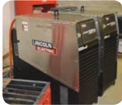
Two Power Wave 1000 SDs are interconnected at the Lincoln Welding Technology Centre allowing twin-wire welding with up to 1 000 A per arc. The units can also be operated in parallel to give a combined current of up to 2 000 A into a single submerged-arc wire.
