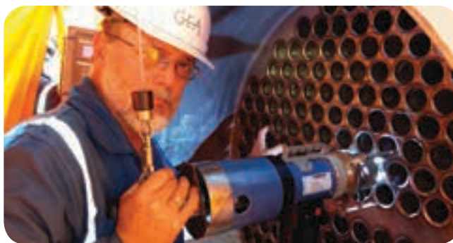
Above: For tube-to-tubesheet welding, Kelvion Thermal Solutions has developed a modified orbital welding technique using copper weld retainers that enables single-pass welding without any overlap into the tube bore. Left: Kelvion Thermal Solutions has developed a way of tube-to-tube welding on serpentine heat exchangers. The method uses filler-metal inserts (inset) to enable an orbital system to be used to complete each weld in a single pass without under filling the joint.
