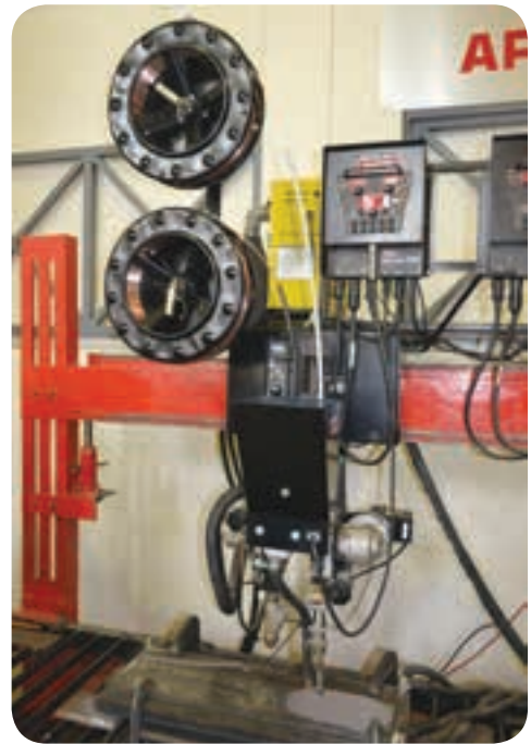
The stick-out extender, which is fitted onto the end of the torch instead of the normal contact tip, raises the electrical contact tip for more resistive heating. Along with the deposition advantages of ac pulsing, stick-out extenders increase deposition rates significantly.
