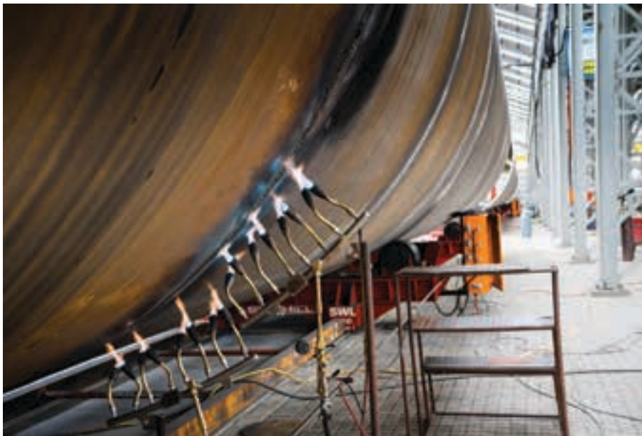
Lindoflamm applications include: pre-heating; maintaining interpass temperatures; post-weld heating; flame straightening; and flame hardening.
