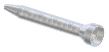
All mixer nozzles are industrial grade safe to 100psi and silicone free plastics. Manufactured from high density polypropylene with white mix elements. Total length of 293mm. The end is stepped with a 4.0 mm hole outlet.
