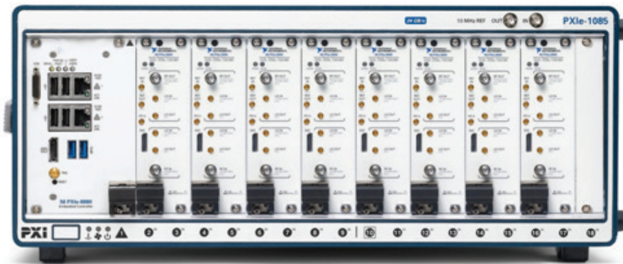
Figure 4. Typical 8x8 MIMO System with 8 VSTs
