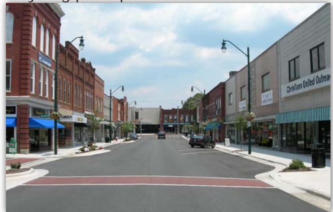
In a Main Street context like that proposed for the civic/cultural/commercial area, on-street parking helps to provide visitors with ready access to stores and buffer pedestrians on the sidewalk from adjacent traffic. (Photo: Ben Hitchings, Town of Morrisville)
