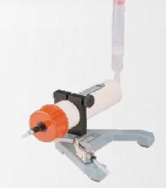
Automatic systems for efficient transfer of materials from cartridge reservoirs to syringe barrels. The filling process is to the bottom end of the barrel which reduces air entrapment and eliminates mess. This range includes an adjustable stand to hold the cartridges which is placed on the workbench with a digital timed dispenser so that each deposit set can be the same. Ideal for repeat syringe filling.
