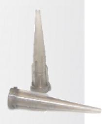
The TE needle series consist of a stainless-steel shaft with a double helix polypropylene hub. This premier line of dispensing needles is burr-free, and electro-polished shaft for unobstructed and consistent material flow. They are silicone and chloride free. For most viscosity fluids and adhesives and safe for use to 100 psi. Supplied in packs of 50, 500 or 1000 tips.
