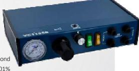
Digital controller for cycling valves by footswitch or via PLC with the I/O port. 3000T controls all pneumatic valves such as pinch tube, diaphragm, needle and spool. 0.001 - 99.99 second timer. Built in timer memory. Highly accurate timer. Operates by footswitch control.
