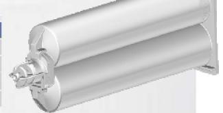
High density bayonet static mixer nozzles for use with A Series twin 50ml cartridges. Stepped at the outlet end for controlled dispensing direct or by using our luer lock tip adapters for higher precision. These mixer nozzles are suitable for most two-component materials. They are constructed of high grade polypropylene. All products are industrial grade and silicone free plastics.
