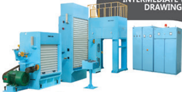
FINE WIRE DRAWING M/C WITH CONTINUOUS ANNEALING M/C
