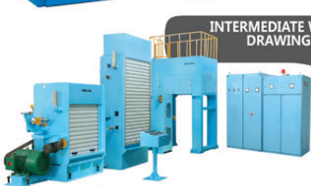
FINE WIRE DRAWING M/C WITH CONTINUOUS ANNEALING M/C
