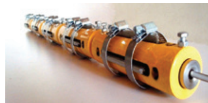
▲ Wire cleaning by BH-S system
