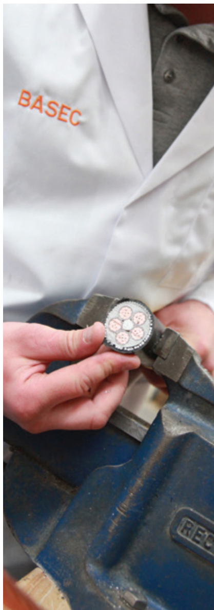
▲ Low and medium voltage cable testing at BASEC
