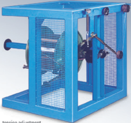
Payoff with dancer accumulator and double pivot to pre-load
