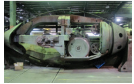
▲ Northampton 1.8m double twist buncher, made in 1995
