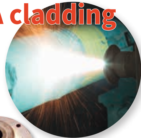
Above: Thermaspray thermal spray coatings reduce erosion damage to components, equipment and systems.
