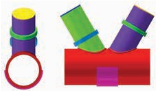
Figure 6: A simplified 3D computer model of a tubular K-joint.
