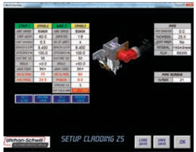
The Hybrid 3D Z5 automatic welding control and data logging system ensures the pre-determined ratio of strip and wire feeding is maintained during H-ESC.
