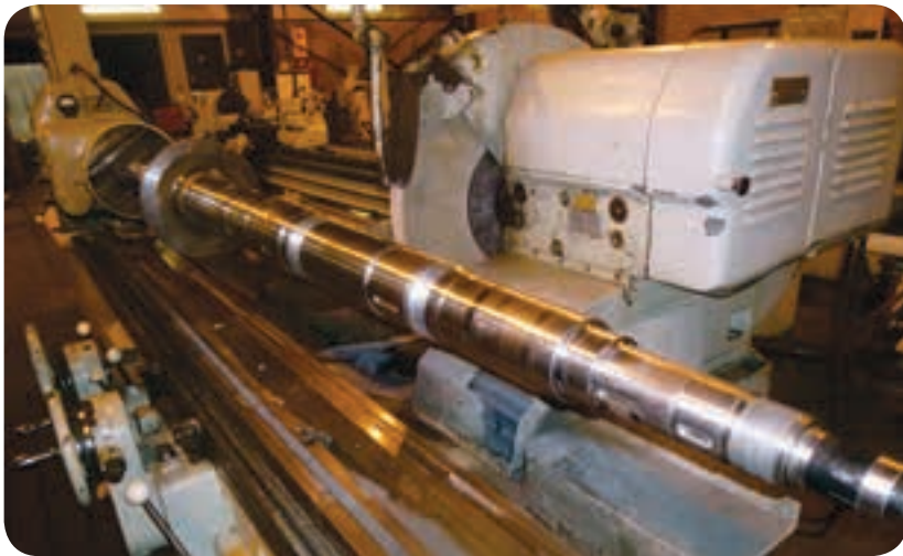
Thermaspray pump refurbishments, completed with business partner (Sulzer), include machining, grinding, thermal spray coating, and final grinding.
