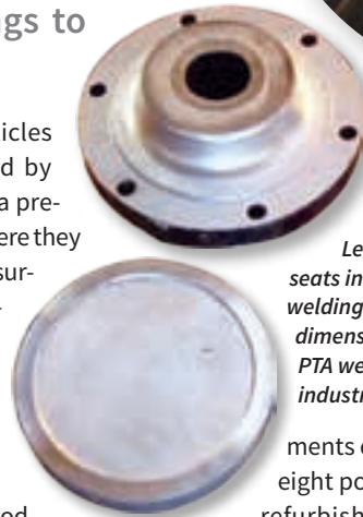
Above: Thermaspray thermal spray coatings reduce erosion damage to components, equipment and systems.
