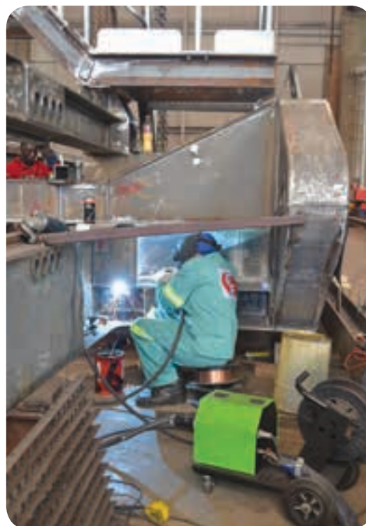
A bulk materials handling system being fabricated in Efficient Engineering’s Phase IV facility in Tunney, Germiston.
