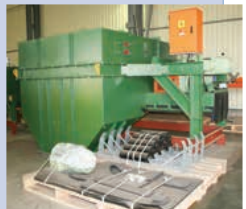
A fully assembled, quality control- and FAT approved Multotec sampler with spares ready for despatch.
