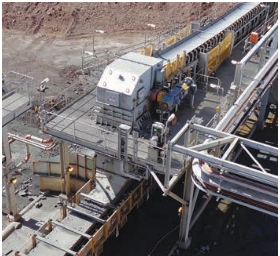
The Weba Chute System is a custom engineered transfer point solution designed to address the numerous issues plants face with material movement.
