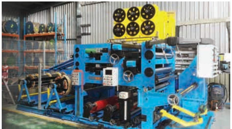
Above: The newly commissioned automatic foil-winding machine at the WTA Wadeville facility.
