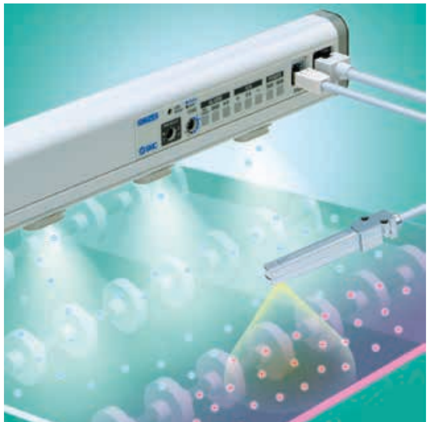
The bar type ioniser is equipped with nozzles, which generate charge, which is blown onto the application. These SMC ionisers can be fitted with sensors able to determine if a positive or negative charge is required. The appropriate charge will be generated accordingly, and in energy saving mode, the system stops generating ions as soon as the charge has been neutralised.
