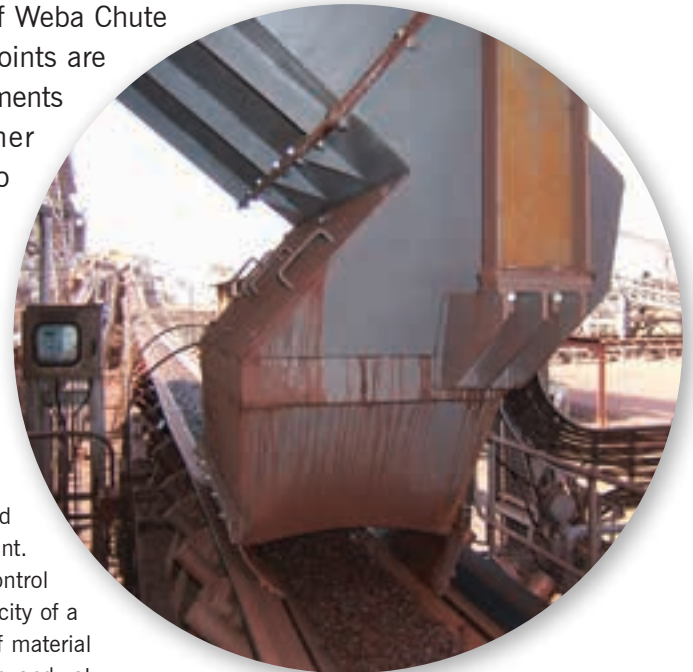
Each Weba Chute System is engineered for the specific application and this is what accounts for the success that these transfer points have achieved worldwide.
