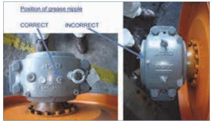
“We have had cases where we have had to move the grease point so that both sides of the spherical roller bearing would be adequately lubricated.
