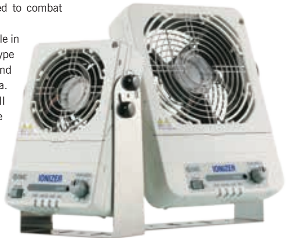
SMC's fan style ioniser eliminates static for bench tops and enclosures. Unlike bar or nozzle types, this fan ioniser does not require a pneumatic air supply. The fan draws in ambient air, then ionises the air with four electrodes located around the perimeter of the discharge grill.
