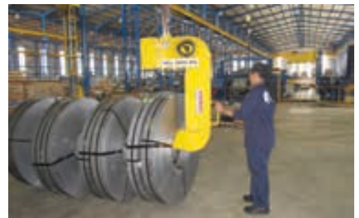
A ‘C’ hook from Elephant Lifting Equipment that is used for lifting steel coils.
