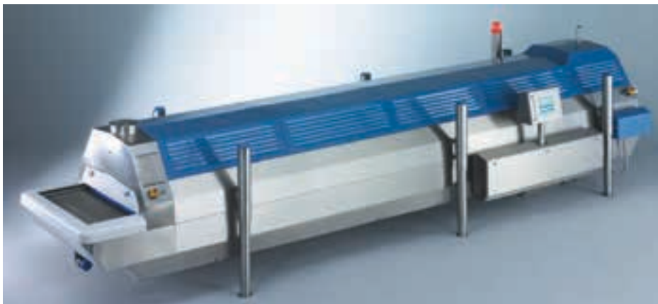
Suited to individual food pieces or ready meals, such as meat patties and fish fillets, Cryoline® MT tunnel freezers are designed to be easy to dismantle and clean, with a stainless steel all-welded construction, internal run-off troughs and smooth and sloping surfaces.
