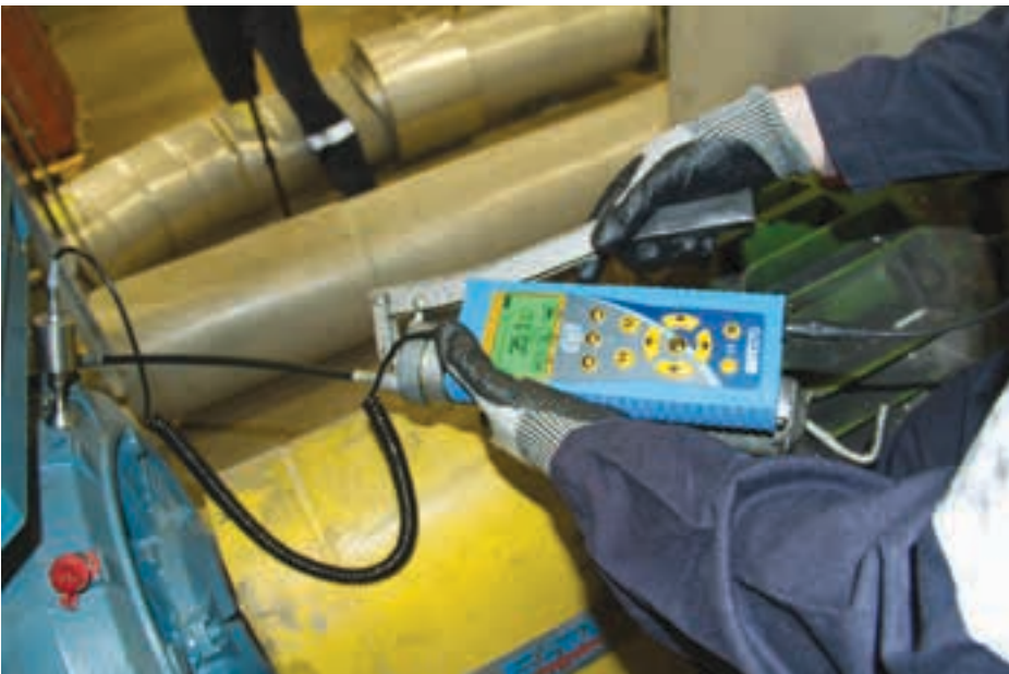
An SDT ultrasound detector is being used here to determine the optimum lubrication level for a bearing. This exemplifies how predictive maintenance tools and techniques can be added to a preventative maintenance strategy to further failure.
