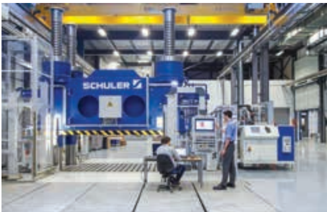
Left: The UK’s National Composites Centre (NCC) has installed the world’s largest openly accessible high rate manufacturing press for composites. Right: The upstroke short-stroke press made by Schuler has a press force of 36 000 kN and a clamping surface of 3.6×2.4 m. From top dead centre, the slide is moved by a drive cylinder to its support position and locked there. Photos courtesy of NCC.
