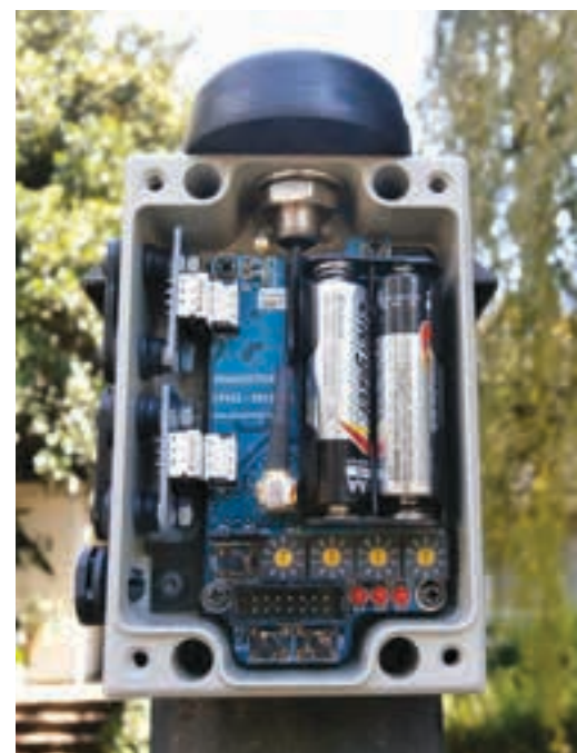
Ernst Pretorius' Draadsitter detects tampering on fences up to 800 m long.
