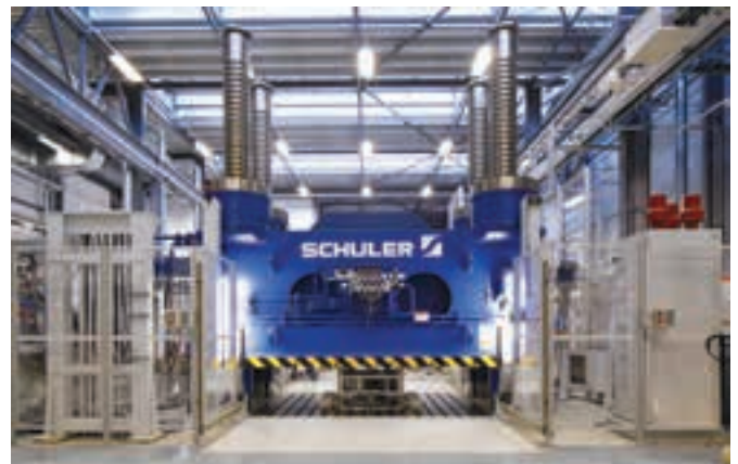
Left: The UK’s National Composites Centre (NCC) has installed the world’s largest openly accessible high rate manufacturing press for composites. Right: The upstroke short-stroke press made by Schuler has a press force of 36 000 kN and a clamping surface of 3.6×2.4 m. From top dead centre, the slide is moved by a drive cylinder to its support position and locked there. Photos courtesy of NCC.
