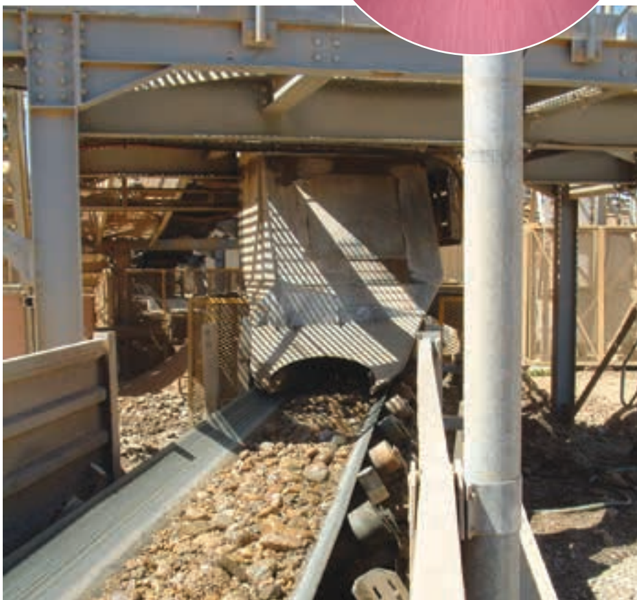
Weba Chute Systems control material movement in such a way as to match the product discharge velocity with the belt speed, completely eliminating or greatly reducing spillage.
