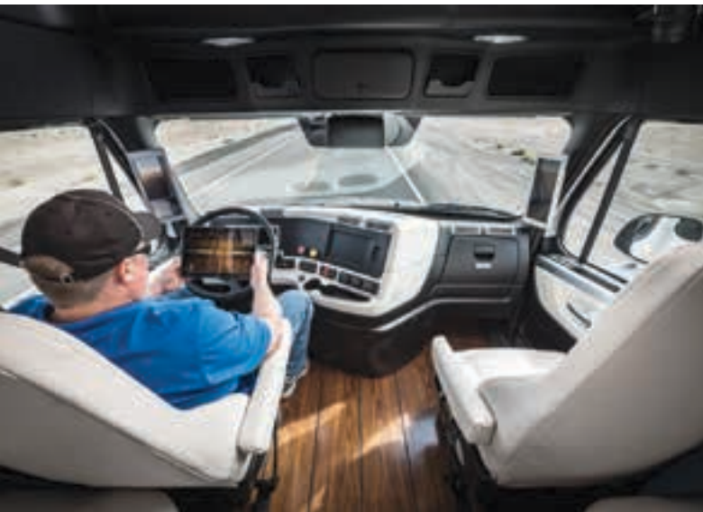
As soon as the truck is safely on the highway, the driver can activate the Highway Pilot system, which uses a complex stereo camera and radar systems with lane-keeping and collision-prevention functions to regulate the speed, apply the brakes and to steer the truck.
