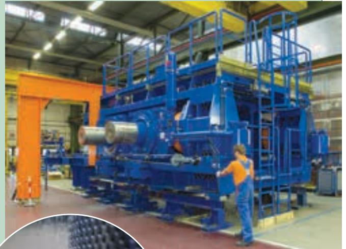
Above: A Weir Minerals HPGR at final assembly stage at the company's manufacturing facility in Venlo, The Netherlands.
