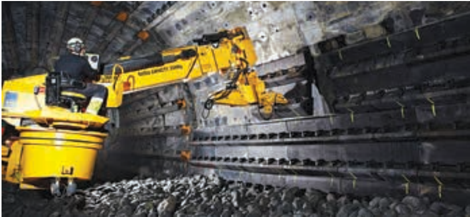
Megaliner is a new, innovative mill-lining concept, dramatically improving worker safety and maximising mill availability. Each liner covers a large area, has few attachment components and a unique attachment system, which provides a safer working environment for the installation crew.
