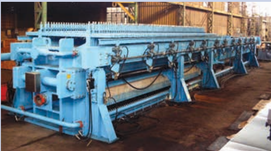
A Shriver® filter press, also supplied by FLSmidth to the Mufulira Smelter, for dewatering concentrate. These industrial grade heavy-duty machines, are designed for long life, low maintenance, easy operation and cost-effective filtration and more than 30 000 have been installed globally.
