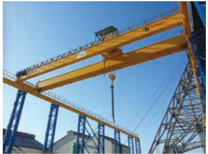
A double girder top riding electric overhead crane.
