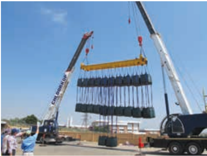
A specially designed 20 t capacity lifting beam for handling sugar bags.
