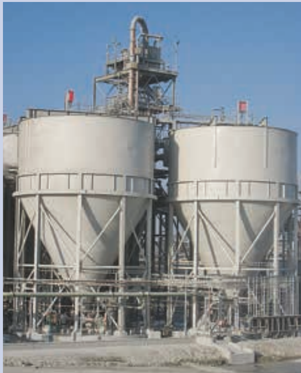
FLSmidth has supplied an Eimco clarifier and thickener (E-CAT) to Mopani Copper Mines in Zambia for its Mufulira Smelter.
