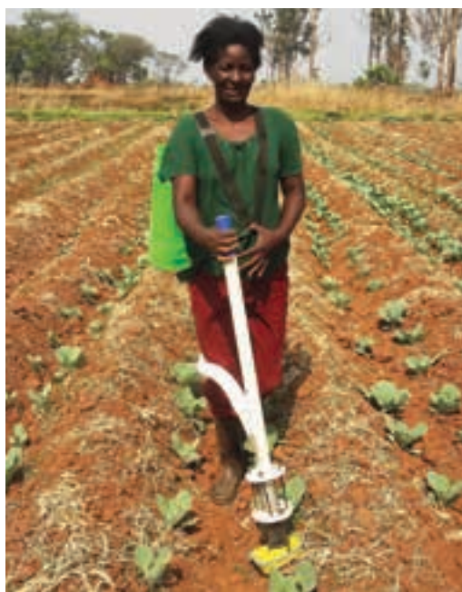
Silwawa's spot fertiliser applicator goes ahead of the walker and inserts fertiliser into the soil while supporting the hand that holds it.
