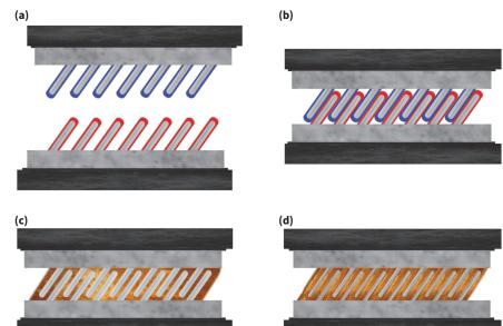
**Fig. 2** — Low-temperature metallic gluing enabled by well separated metallic nanorods: (a) Two sets of well separated nanorods, which have metallic cores and shell elements that form a eutectic alloy, are brought together, (b) they interpenetrate under fingertip pressure, (c) shell elements meet and form a eutectic alloy, which is liquid at room temperature, and (d) mixing of eutectic liquid with a metallic core leads to formation of three-component alloys that are solid at room temperature.
