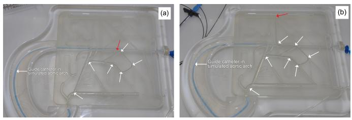
**Fig. 6** — Testing of LRM full guidewire 0.014-in. diameter in 2D plate model. Hypotube joint (a) and LRM solid-state weld joint (b).
