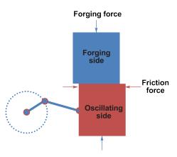
Fig. 1 — Mechanical LFW schematic.
