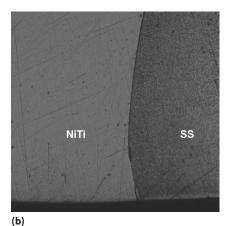
**Fig. 1** — Post polishing SEM image of joint shows its seamless nature (a); SEM image of joint after etching shows presence of small grains in HAZ (b).
