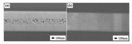
**Fig. 4** — Metallic glue formed in air and under a small pressure of 9 MPa (a) at room temperature, and (b) at 100°C. Reprinted with permission from *Scientific Reports*<sup>[15]</sup>.
