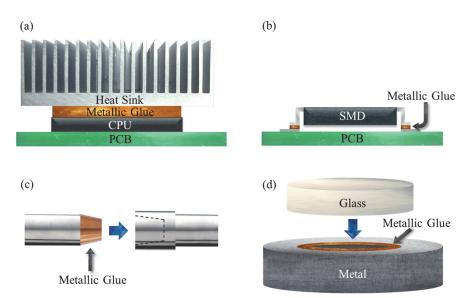
**Fig. 1** — Various applications of metallic glue: (a) A central processing unit (CPU) on a printed circuit board (PCB) connected to a heat sink, (b) a surface mount device attached to a PCB, (c) a press-fit pipe fitting for environments where welding is dangerous or impossible, and (d) a glass plate attached to metal with a different coefficient of thermal expansion to cover a cavity with a hermetic seal.
