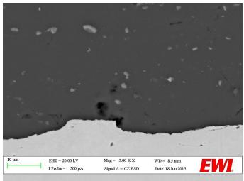
Fig. 5 — Aluminum-to-steel interface under high magnification using SEM.
