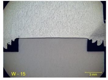
Fig. 4 — Cross-section of aluminum-to-steel joint.
