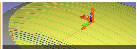
AFP layup flaws are displayed against the programmed layup, color-coded by feature type for rapid disposition and rework. Courtesy of Flightware.
