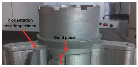
Fig. 6 — As-manufactured part with build pause visible.
