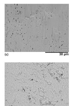
**Fig. 5** — SEM image of fracture surface, post tensile testing. Low magnification (200×) of hypotube joint and LRM solid-state joint, respectively (a) and (b); high magnification image (2000×) of NiTi wire side of hypotube joint and LRM solid-state joint, respectively (c) and (d).
