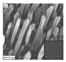
Fig. 3 — Scanning electron microscope image of well separated Cu nanorods. Courtesy of X. Niu, et al., *Phys. Rev. Lett.*, Vol 110, 136102, 2013.
