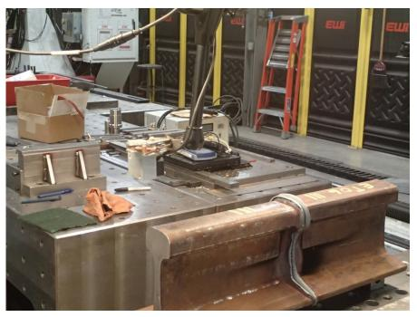
Fig. 7 — Full-section rail joined by LFW.
