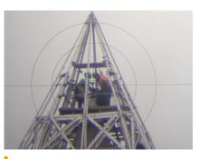
Top view of the monument via the total station surveying tool, captured by placing a smartphone camera near the eyepiece. Courtesy of NOAA.
