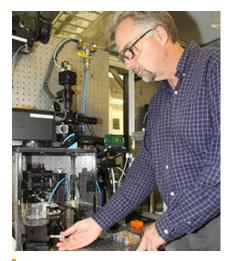
LLNL optical engineer Bryan Moran makes an adjustment to the Large Area Projection Micro Stereolithography machine. Courtesy of Steve Wampler/LLNL.
