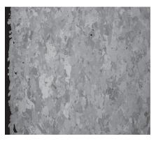
**Fig. 4** — Typical microstructure of a HIP'd specimen. Courtesy of NASA.
