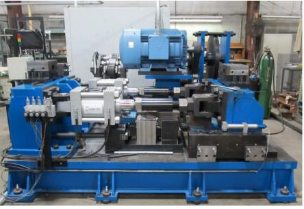
Fig. 6 — 150-ton mechanical LFW system.
