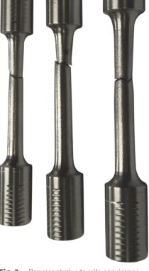
Fig. 3 — Representative tensile specimens after testing.
