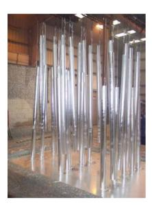
Although powder painted and unprotected steel can last for many years when submerged or buried, it must be FULLY covered, inside and out. Left unprotected, steel will react with its surrounding environment and revert to oxide compounds (rust), thus consuming the pier in the process.
