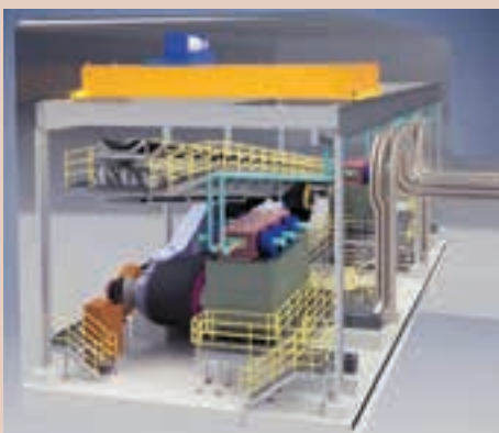
3D rendering of the Oyu Tolgoi underground drive chamber for one of the four slope conveyors with 2 x 5,5 MW gearless drives.
