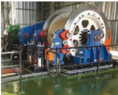
A single drum service winder provided to a mine by Tech Edge.
