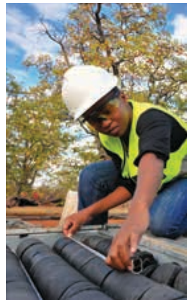
Core logging at the Makhado project (photo: CoAL).
