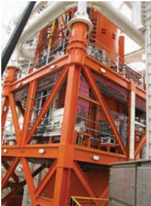
A from-the-deck view of the Seabed Tool (SBT), a world-first advanced sub-sea sampling system aboard the mv SS Nujoma.
