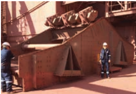
Kwatani management on site inspecting a screen which is en route to the OEM for refurbishment.
