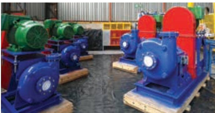
Becker Mining SA has recently supplied five HS pumps to a new furnace slag granulation process plant.
