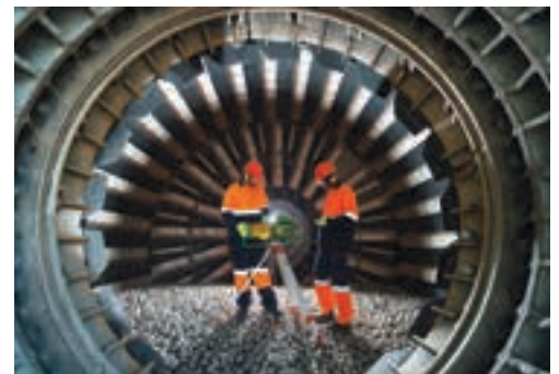
MultoScan, from Multotec Rubber, can accurately measure a mill's liner profile and predict the point at which the mill will start becoming inefficient.
