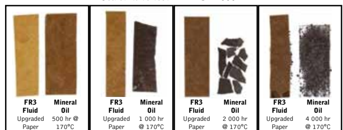
Figure 2: Thermally upgraded papers aged in FR fluid and mineral oil for varying times at 170°C.
