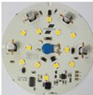
Figure 5. Minimum component count (excluding LEDs) 23 vs 62...one board vs two and the SMPS' second board is two-sided board
