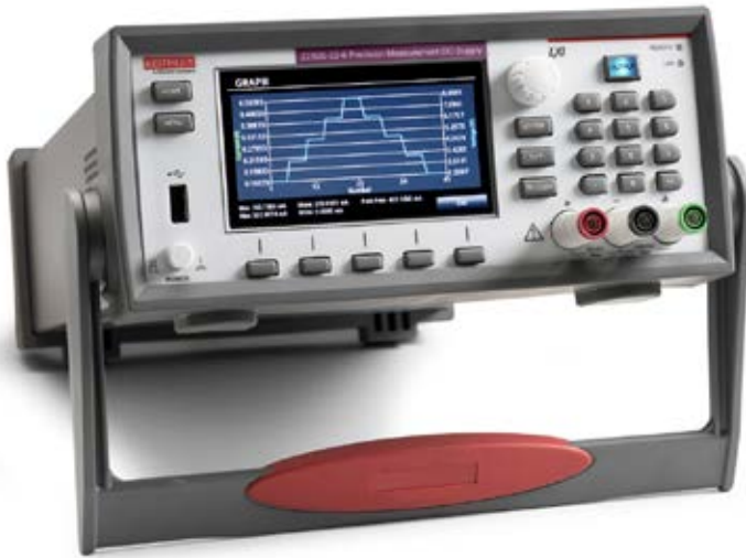
Figure 3. Keithley's Series 2280S Power Supplies can characterize small load currents with 10nA resolution and measure up to 6A very accurately. Four load current measurement ranges—10A, 1A, 100mA, and 10mA—allow measuring both full load currents and standby/sleep mode currents with 6 1/2 digit resolution. It can also capture dynamic load currents as short as 140µs.
