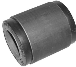
Bushing, Beam End Rubber; 2 1/2" I.D. x 4 3/8" O.D. x 5 1/4" Lg.; Model RT340
