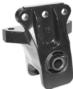
Hanger, LH Shackle; 10 1/2" Frame; Model Airtek
