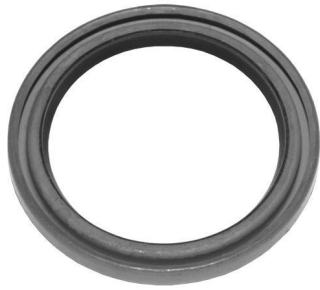
Seal; 2" I.D. x 2 5/8" O.D. x 1/4" Thk.; Included in 334-995 Equalizer Shaft and Bushing Assy.; Model "Parallelogram"
