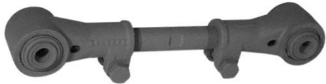
Torque Rod, Adjustable; 15"-17 1/4"Lg.; Includes 321-153 Bushings; Model Q-TR/QS/QT/QU
