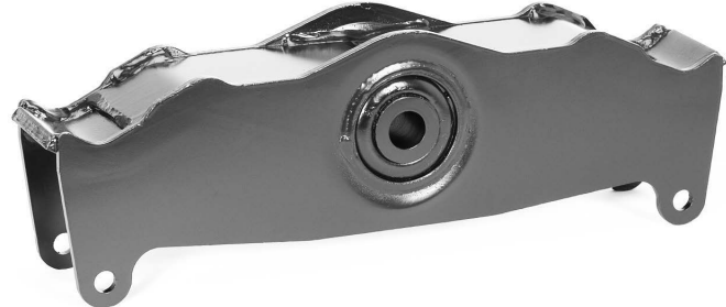
Equalizer Assembly, Fabricated; 21" OAL; Incl. 321-221 Bushing; 53.5/54.5" Axle Spacing; Replaces 338-1717; Models 7600/7650/9600
