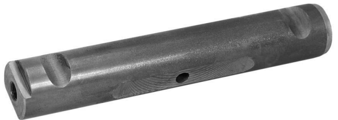
Spring Pin; 1 1/4"OD x 7 7/16"Lg. x 5 3/4" C/C; Front of front; Model 357/379 SBA w/cast eye
