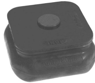
Insulator, Offset; 3 3/4" Thk. x 6" W x 6" Lg.; 1 3/4" Dowel; 70 Durometer, Rubber
