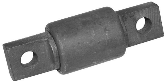
Bushing, High Confinement; Replaces RB-205; Model FASII Airliner (Current Production)
