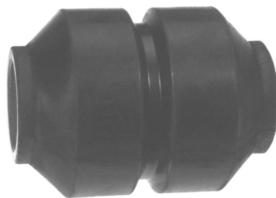
Bushing; 1 1/2" I.D. x 3 1/4" O.D. x 5 1/4" Lg.; 70-75 Durometer; Model RSS235
