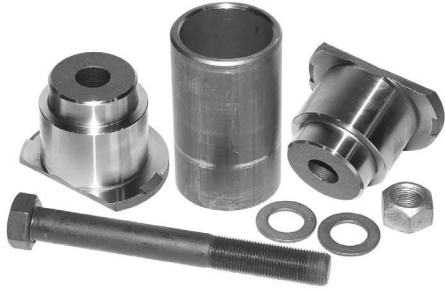
Adapter Kit, Solid Adapters; Use w/321-126 Bushing (5 3/4"); Model RT340 - 400
