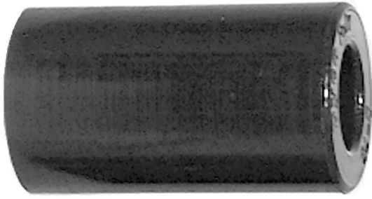
Bushing, Urethane; 7/8"ID x 1 1/2"OD x 2 3/4"Lg.
