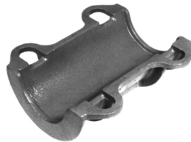
Trunnion, Upper Half; Underslung; Model Straddlemount Trailer Single Point
