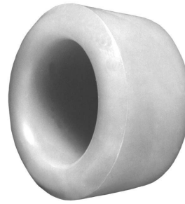
Bushing, Urethane; 1 3/8" I.D. x 2 3/16" O.D. x 1 13/16" Lg.; OE Cast Rods Only; Model FH34A-44A
