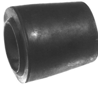
Bushing, Torque Rod; 2 3/16" O.D. x 1 1/4" I.D. x 1 3/4" Lg.; Included in 334-565 Bolt and Bushing Assy.; Models F, J, NF-2, NT-2, NT2W
