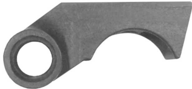
Bracket, Torque Rod Seat; 5" Round Axles; HEIGHT = 1 3/4"; Use w/ 334-252 T/R Bolt and Bushing Assy.; Model 21B
