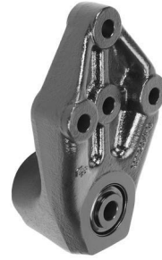
Hanger, Shackle; Incl. RB-233 bushing; Models Columbia, Coranado, Cascadia, Argosy, Condor
