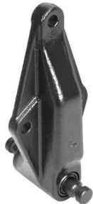
Hanger, Shackle; Incl. RB-249 bushing; Front
