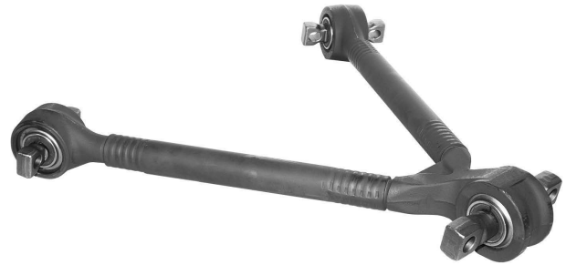
V-Rod; Front of Rear; 54" Axle Spacing; 25.8" Legs; Model Tuftrac, 40K
