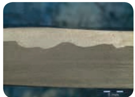
Micrographs of the STELLOY-clad layer for three different welding positions: left, from the overhead position; centre, from the 3:00 vertical up position; and right, from the downhand position.
