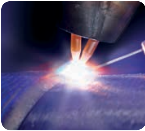
TIG er technology involves the juxtaposition of two TIG arcs, organised, controlled and combined to act as a single arc, with the addition of wire heated by a third power source.
