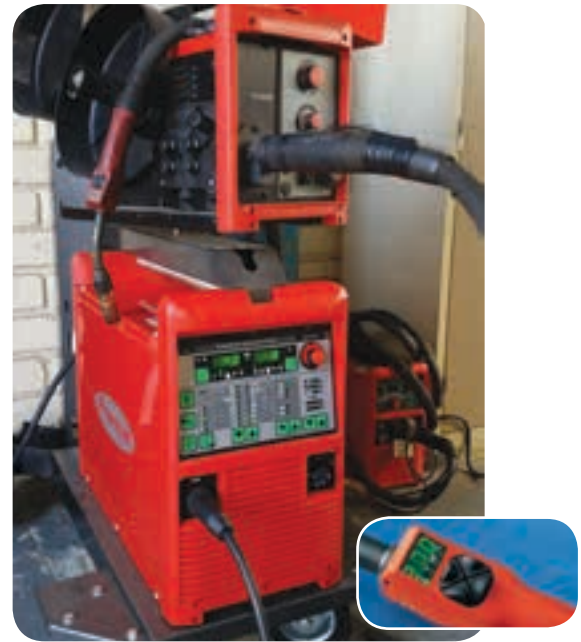
Fronius' Transpuls (TPS) inverter and the VR4000 wire feeder – along with the Job-master torch with its integral remote control and weld data display – are pre-programmed to enable out of position, in-situ welding of the all common cobalt-based alloys.
