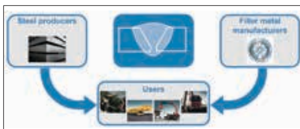
Figure 1: Conventional weld design. Filler metals and base materials are usually developed separately and offered independently from each other.
