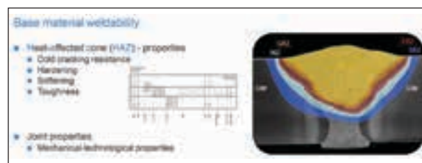
Figure 3: Characterisation of the base material weldability primarily focuses on the properties in the heat-affected zone (HAZ) – cold-cracking resistance, hardening, softening and toughness.
