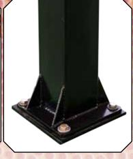
4 SUPPORT GUSSETS •WELDED GUSSETS ELIMINATE POLE SWAY & LESSEN VIBRATION. •SLOTTED BASE PLATE HOLES ALLOW ADJUSTMENT TO SQUARE THE POLE TO THE DRIVEWAY OR COURT.
