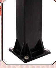
8 SUPPORT GUSSETS •WELDED GUSSETS ELIMINATE POLE SWAY & LESSEN VIBRATION. •SLOTTED BASE PLATE HOLES ALLOW ADJUSTMENT TO SQUARE THE POLE TO THE DRIVEWAY OR COURT.
