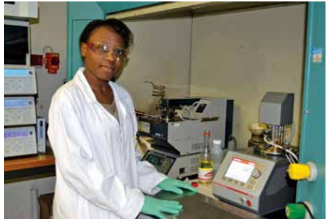
Senior laboratory technician at WearCheck, Lizzy Chabangu, operates the condition monitoring company's brand new PMA5 Pensky Martens closed cup flashpoint tester in Johannesburg recently.
