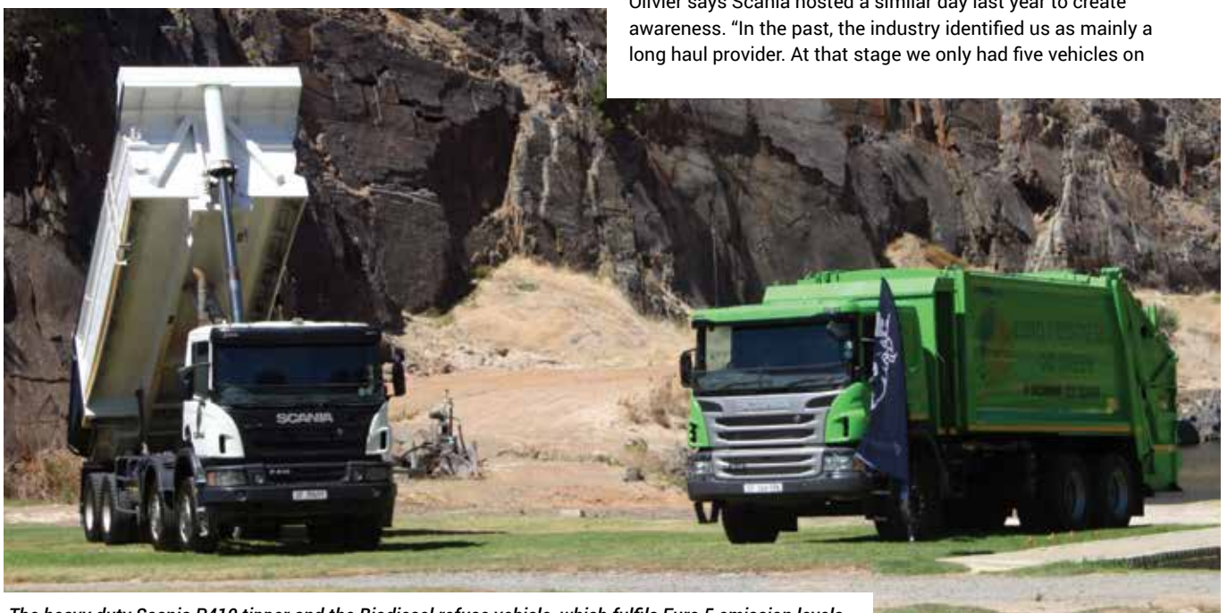
The heavy duty Scania P410 tipper and the Biodiesel refuse vehicle, which fulfils Euro 5 emission levels.
