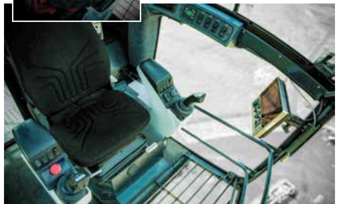
The new Potain Topless cranes are equipped with Manitowoc's Crane Control System, or CCS which helps contractors get work done faster and with greater precision.
