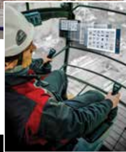
The new Potain Topless cranes are equipped with Manitowoc's Crane Control System, or CCS which helps contractors get work done faster and with greater precision.
