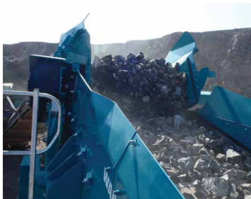
The Powerscreen Warrior 1400XE – powered by a Premiertrak 600 jaw crusher.
