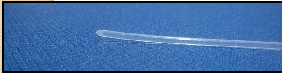
MR markers for CT/MR applicator. They are filled with water. \text{CuSO}_4 can also be used.
