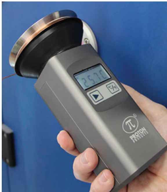
○ The new HTG400 handheld wire temperature gauge from Proton Products
