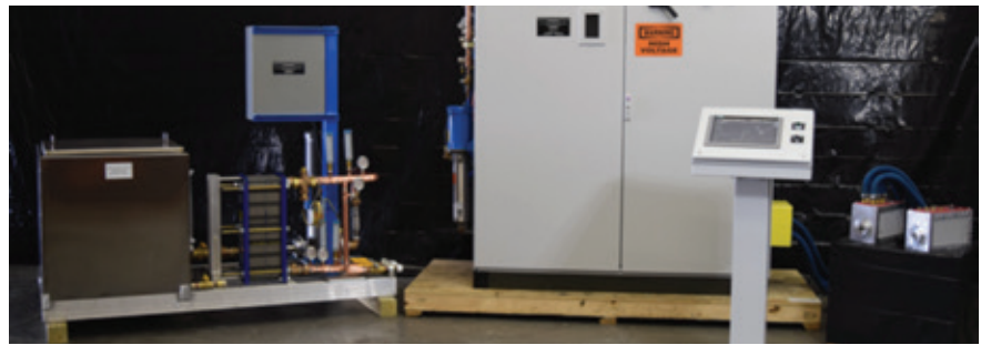
○ MHD power supply, coils and cooling system
