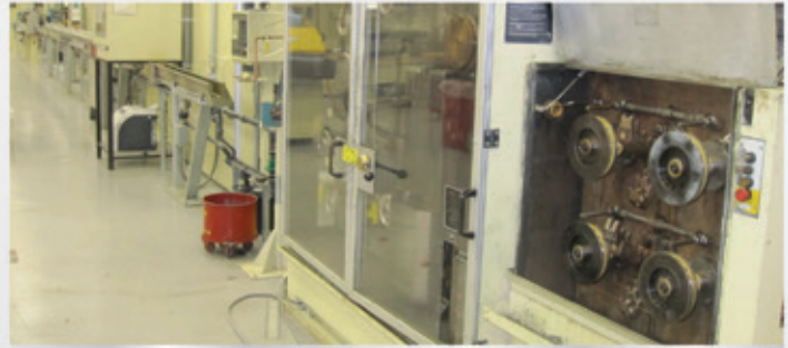
60mm Nokia/Niehoff Tandem Wire Insulating Line
