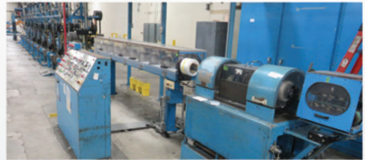
Tensor SZ Cabling Line
