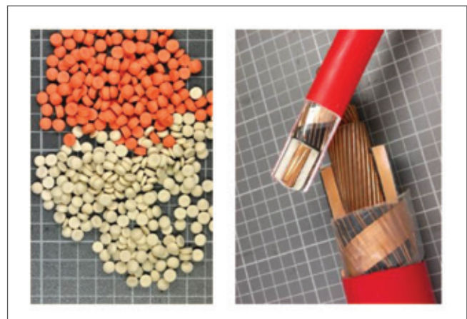
○ Figure 1: MV insulation containing lead (orange) and lead-free (white), from pellets to cables
