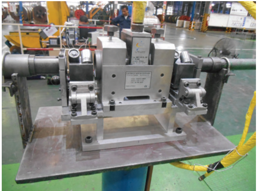
○ The eddy current system from CMS
