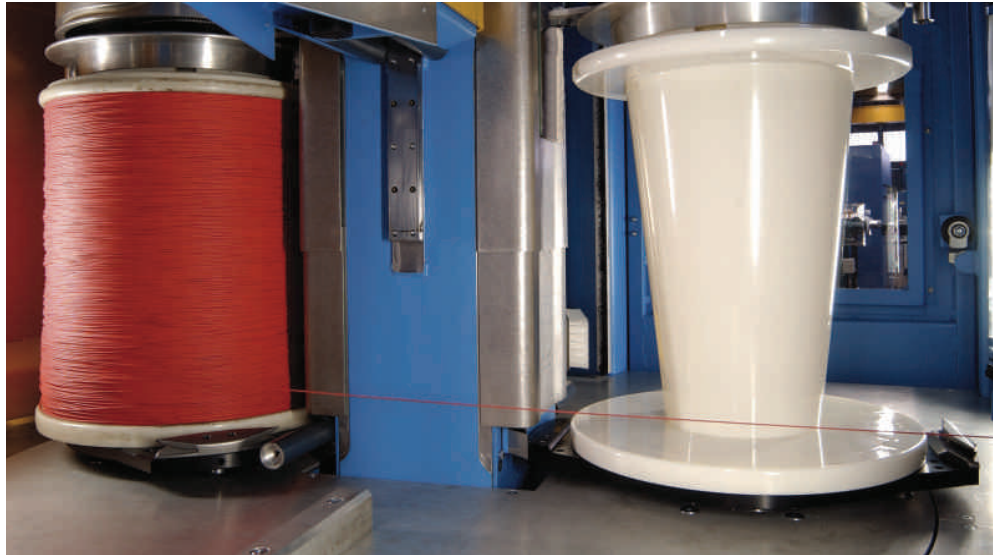
▲ Automatic change of NPS spools at full speed on the new generation double spooler SV410D
