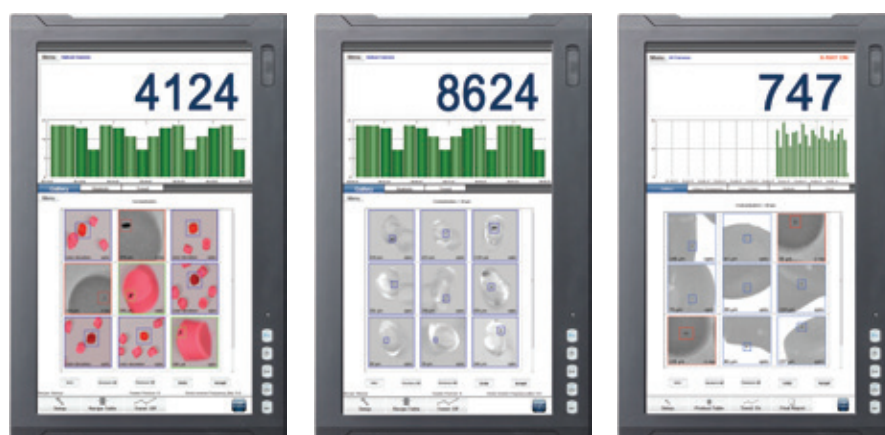
Visualisation, on the Ecocontrol 6000, of detected colour deviations; contamination inside transparent pellets; and contamination inside the pellets and on their surface
