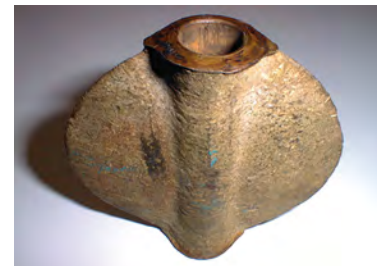
Uniform attack corrosion over the entire surface of a cupro-aluminium valve disc
