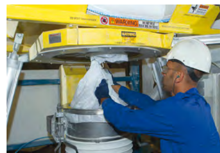
The operator connects the spout to a Spout-Lock™ clamp ring, which is mounted atop a Tele-Tube™ telescoping tube.
