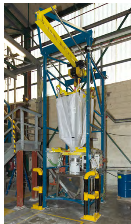
Automated, safe, and dust-free, the Flexicon discharger is equipped with an integral flexible screw conveyor.
