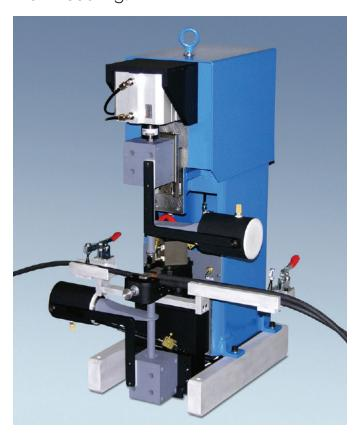
Sonobond's Wedge-Reed system uses a vertical, vibrating reed, driven by a wedge-shaped coupler and transducer assembly. With the line of static clamping force directly above the parts to be welded, high clamp force is achieved without bending stress or stalling. The tin coating is dispersed, and the copper wire is welded without impairing the conductivity of the copper.
