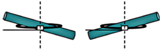
Figure 7: Orthogonality effect. Primary conductor position versus the axis of the Rogowski loop.
