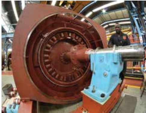
Alpheus Mtshali, from Marthinusen & Coutts, with the 1 586 kW 187,5 rpm, 3 300 V, 278 A stator.
