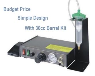
Air Output: Air Input: Timer: Timer Display: Power: Cycle Initiate: Timer Repeatability: Timer Frequency: Dimensions: Weight: Standards: Warranty: 0-100 PSI 80-100 PSI 0.01 to 30 Seconds (Adjustable) n/a 220V AC Foot switch or finger switch +/- 5% Up to 550/minute 235 x 225 x 64mm 2.2kg CE approved 1 Year
