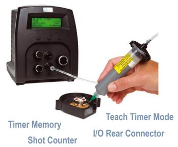
Air Output: Air Input: Timer: Timer Display: Power: Cycle Initiate: Timer Repeatability: Timer Frequency: Dimensions: Weight: Standards: Warranty: 0-100 PSI 80-100 PSI 0.008 to 60 Seconds (Adjustable) LCD 110/ 220V AC Foot switch or optional finger switch +/- 0001% Up to 600/minute 152 x 165 x 178mm 1,2kg CE approved 1 Year
