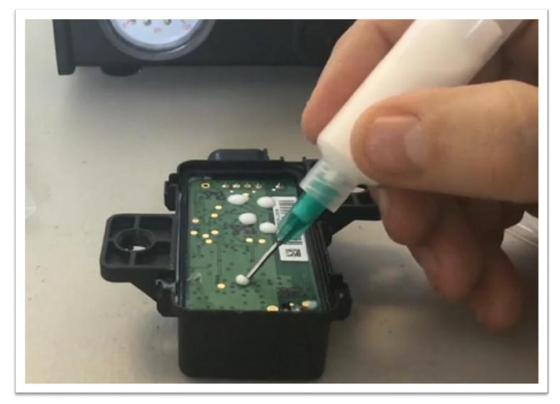
Bench top, air-powered dispensers for most adhesive and paste applications. Featuring an adjustable 0-100 psi air regulator for setting flow rates when dispensing most low, medium and high viscosity materials. A low pressure 0-15 psi version is available for dispensing very watery liquids, cyanoacrylates or solvents. All air powered dispensers use a three way air valve for quick shut-off or air to prevent fluid oozing from the tip when the foot pedal is released. Fast shut-off each time.
