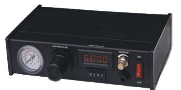
LED Display Teach Timer Mode Choice of Barrel Size Air Output: Air Input: Timer: Timer Display: Power: Cycle Initiate: Timer Repeatability: Timer Frequency: Dimensions: Weight: Standards: Warranty: 0-100 PSI 80-100 PSI 0.01 to 99.99 Seconds (Adjustable) LED 220V AC Foot switch or finger switch +/- 0005% Up to 600/minute 246 x 145 x 65mm 2.9kg CE approved 1 Year
