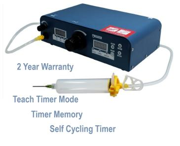
Air Output: Air Input: Timer: Timer Display: Power: Cycle Initiate: Timer Repeatability: Timer Frequency: Dimensions: Weight: Standards: Warranty: 0-100 PSI 80-100 PSI 0.01 to 99.99 Seconds (Adjustable) LCD 110/ 220V AC Foot switch or finger switch +/- 0005% Up to 600/minute 220 x 210 x 67mm 3.5kg CE approved 2 Years
