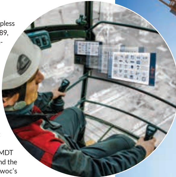
Above: The new Potain Topless cranes are equipped with Manitowoc's Crane Control System, or CCS.
