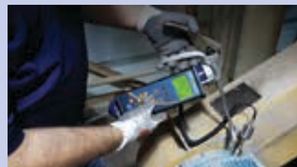
LUBExpert® is an on-board lubrication and greasing assistant that uses ultrasound technology.
