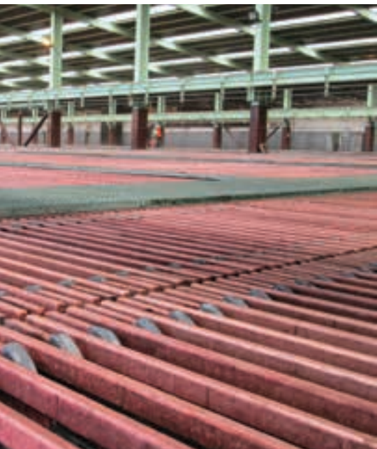
Above: A Jameson flotation cell in operation at Lumwana in Zambia. The system offers the highest possible throughput in a very small footprint, with froth washing maximising the concentrate grade in a single flotation stage. Left: IsaKidd Technology, shown here in use at the Kamoto Copper Company (KCC) in the DRC, is the global benchmark in copper electrowinning accounting for over 11 mtpa of copper production from over 100 licensees.
