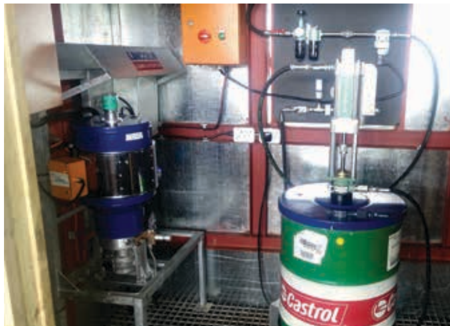
The Lincoln Quiklube P203 progressive system can deliver significant savings at sugar mills.
