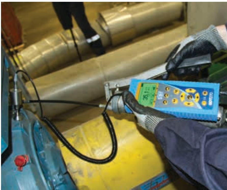
By coupling vibration analysis with an actively managed lubrication programme involving measuring friction during the greasing process and periodically in service using an ultrasonic detection system, blind greasing with fixed quantities at fixed intervals could be replaced with the application of an optimum quantity of grease at the times when needed.
