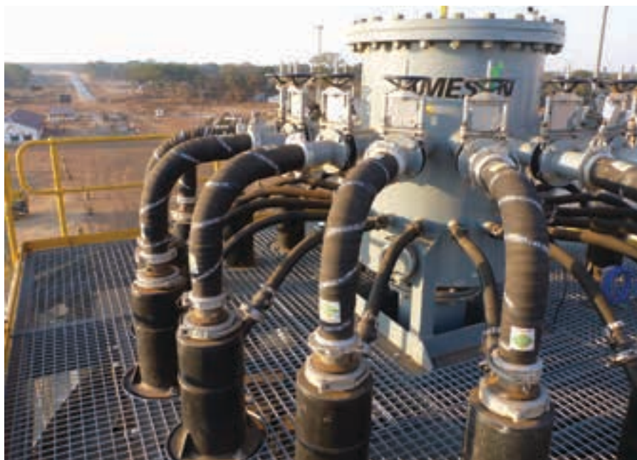
Above: A Jameson flotation cell in operation at Lumwana in Zambia. The system offers the highest possible throughput in a very small footprint, with froth washing maximising the concentrate grade in a single flotation stage. Left: IsaKidd Technology, shown here in use at the Kamoto Copper Company (KCC) in the DRC, is the global benchmark in copper electrowinning accounting for over 11 mtpa of copper production from over 100 licensees.
