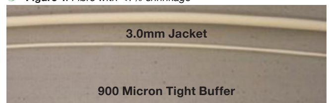
○ Figure 2: Fibre with >4.5% shrinkage
