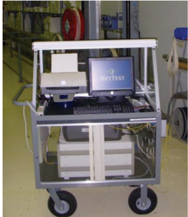
○ Figure 5: Optical Fibre Strain Gauge Measurement System
