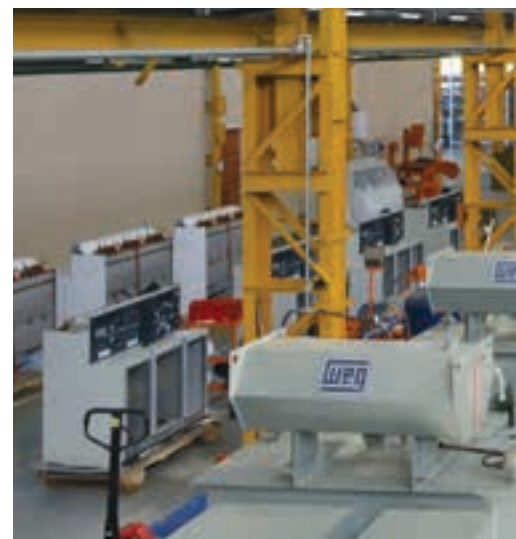
Transformers and ring main units on the production line at WTA Wadeville.
