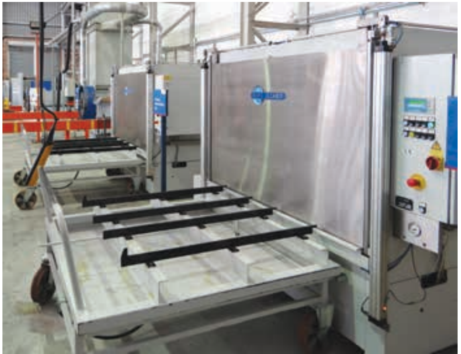
Above: At the starting point of bearing remanufacture are the washdown stations.
