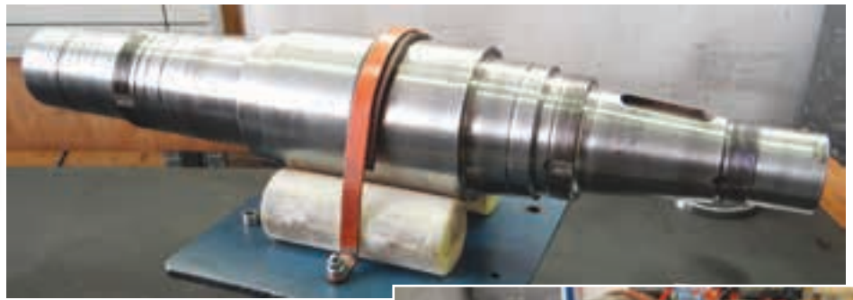
Above and right: Another highly specialised capability of SKF's application engineering team is spindle remanufacture, customisation or redesign for machine tools such as lathes and milling machines.
