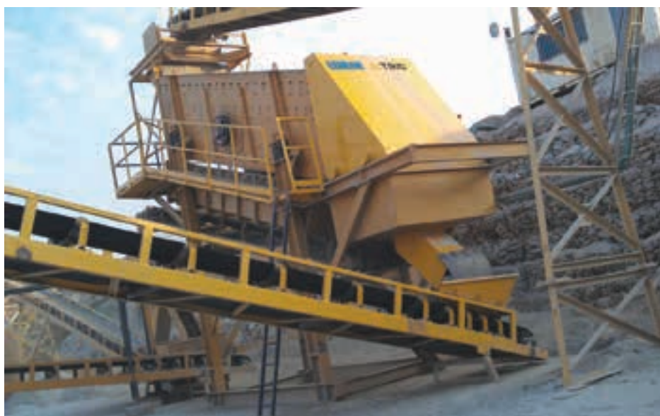
A Trio inclined vibrating screen installed in an aggregate application.
