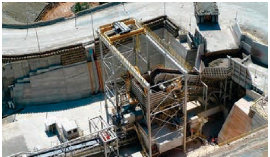
Thyssenkrupp's cost-effective in-pit semi-mobile crushing plants (SMCP) are well suited for coal and ore applications and can lead to significantly reduced operating and capital expenditure (opex and capex).
