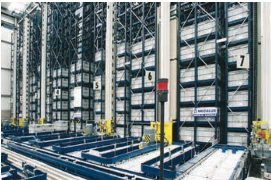
Mecalux develops automatic storage systems for boxes or trays integrating the shelves, machinery and warehouse management software into one single product.
