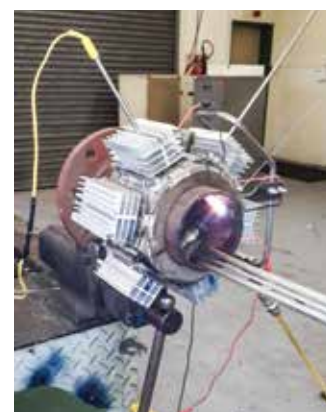
Figure 5: Thermoelectric generator unit simulated test.
