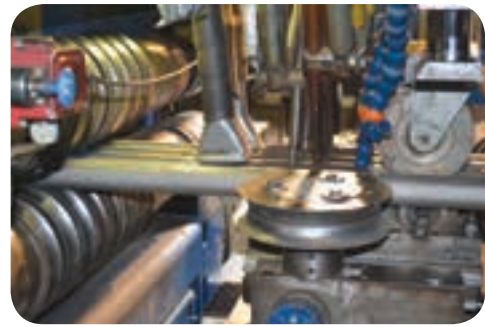
A Pemamek water wall panel being set up for fabrication at Steinmüller’s Pretoria West facility. Pema automatic welding systems were installed by several South Africa-based fabricators for producing membrane wall panels for the Medupi and Kusile boilers. (photographed in 2013).
