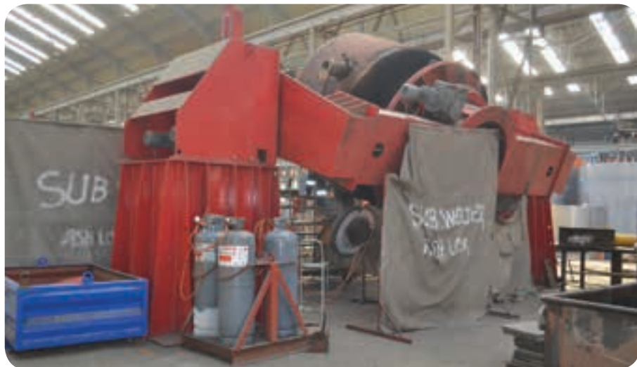
Above and right: The manipulators for refurbishing ashlock vessels consist of rotators with a capacity of 50 t. An internal boom system is synchronised to deposit a spiral weld of equal thickness and heat input across the varying diameter of the conical vessel.
