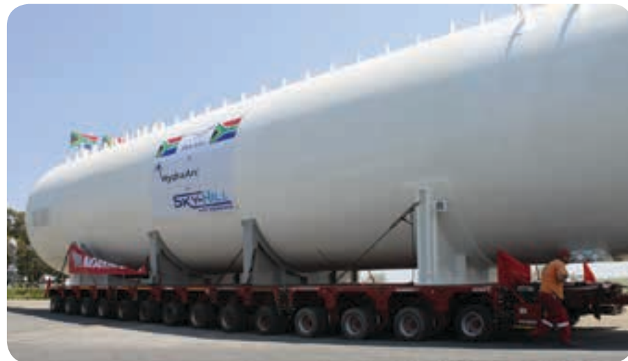
One of five propylene storage vessels manufactured at Sky-Hill. Called bullets, these vessels have a mass of over 446 t, are 59.09 m long with an internal diameter of 6.0 m and a wall thickness of between 45 and 50 mm.
