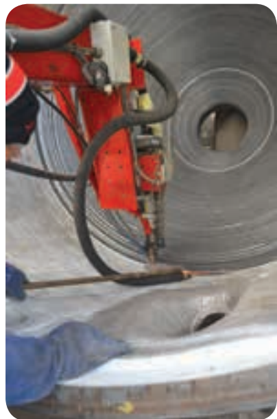
Above and right: The manipulators for refurbishing ashlock vessels consist of rotators with a capacity of 50 t. An internal boom system is synchronised to deposit a spiral weld of equal thickness and heat input across the varying diameter of the conical vessel.
