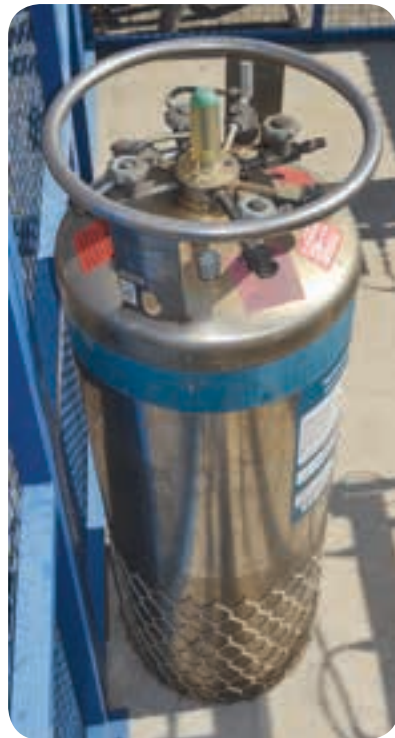
Air Products’ CryoEase solution is an argon liquid offering utilising 600 litre to 2 000 litre maxitanks to service larger welding accounts.
