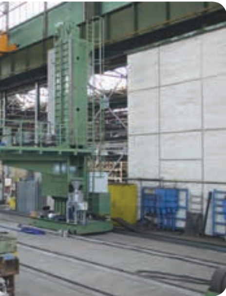
1: External longitudinal welding using a traditional Kistler/Bode column and boom.
