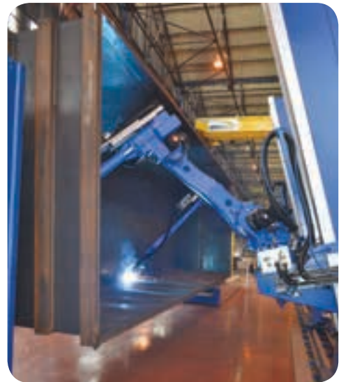
Yaskawa continues to dominate the rail manufacturing industry in South Africa. Shown here is the final wagon welding station at Transnet Rail Engineering (TRE), Bloemfontein.
