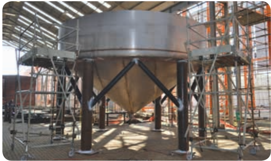
Water tanks for provincial governments around South Africa are made in 3CR12 ferritic stainless steel and using a modular construction that enables them to be easily transported to site, rapidly assembled and welded.
