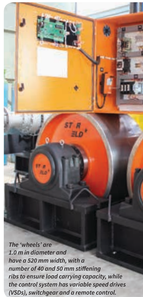
For the driven rolls, Bonfiglioli 7.5 kW induction motors connected to 311 planetary drives on a torque arm were chosen in a simple in-line design.
