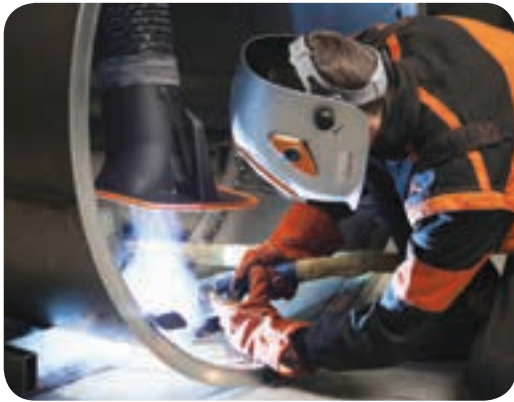
The Kemper autodark 760 has the best possible optical filter classification – Level 1 in terms of the optical quality, light diffusion, homogeneity of the field of vision, and angle dependence.
