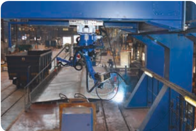
Three new gantry-based welding stations have been installed recently, two in Durban and one in Koedoespoort, to fabricate locomotive bogey. Like this one, each gantry has two robots with manipulators, SKS power sources and Servo Robot vision seam tracking systems.
