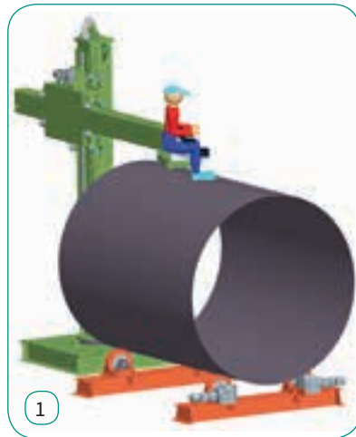
1: External longitudinal welding using a traditional Kistler/Bode column and boom.
