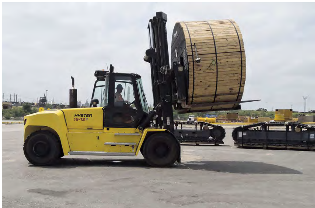
Hyster tyre handlers have become an industry standard for handling and changing tyres on mining and construction equipment fast, efficiently, cost-effectively and safely.
