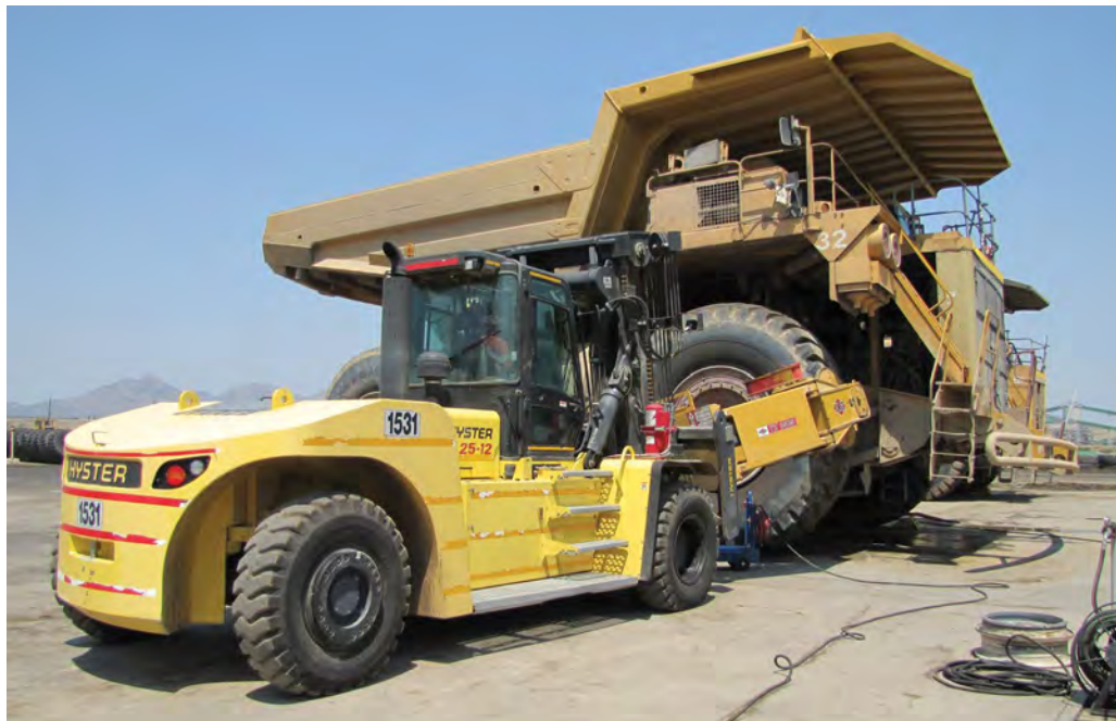
Hyster tyre handlers have become an industry standard for handling and changing tyres on mining and construction equipment fast, efficiently, cost-effectively and safely.
