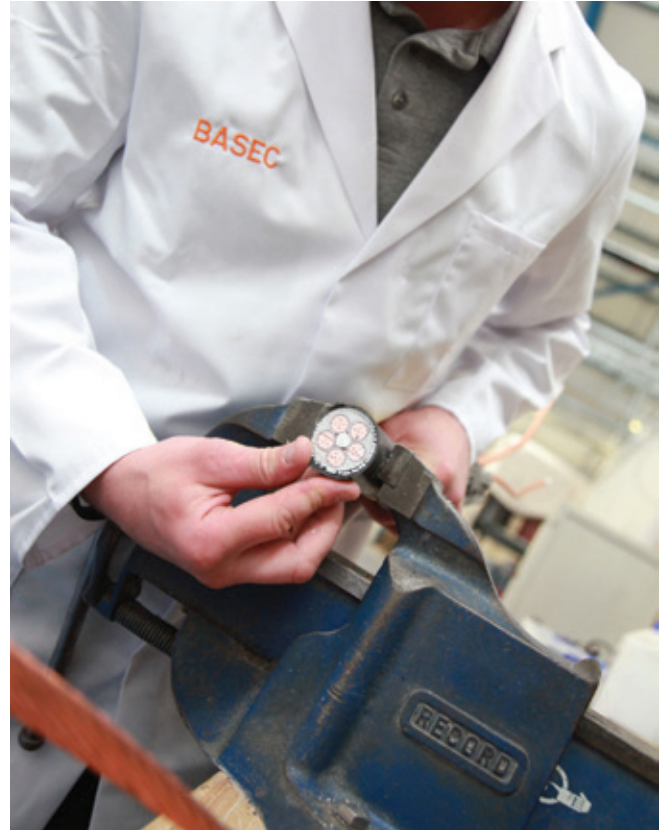
○ Low and medium voltage cable testing at BASEC
