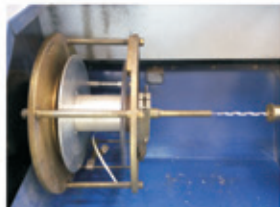
Concentric core horizontal type taping machine (Suitable for barreled tape)
