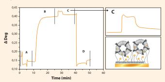
Lipid vesicles are bound to a hydrogel sensor surface and the interaction with a protein is studied. (A) Sensor cleaning injection, (B) Vesicle binding to surface, (C) Protein interaction, (D) Sensor regeneration.
