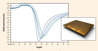
Single monolayer of graphene was measured as 3.5 Å thick at 670 nm wavelength. Thin layers form a single peak in a MP-SPR scan.
