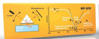
Goniometric arrangement Typical range 1.0-1.4 of bulk RI Wide angular range (up to 38 degrees)
