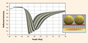
Functionalized gold nanoparticles (50 nm) interacting with a self-assembled polymer layer. Measured at 785 nm.
