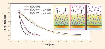
Perphenazine drug release from a micrometers-thick EUDRAGIT® polymer matrix. Faster release rates obtained by adding PVP polymer and varying thickness of the film.
