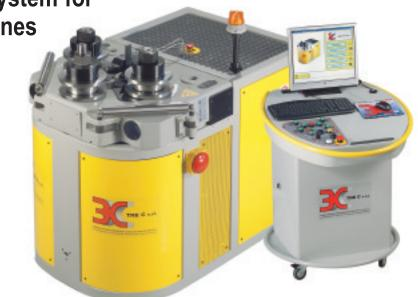
Tre C's CNW333 numerical control system, alongside one of the company's bending machines
