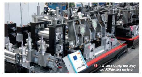
are automatically performed by means of central adjustment drives that are activated by computer control. Adjustments in the forming and sizing section are carried out within minutes, and tool settings as well as other key operational parameters are visualised by digital displays.
