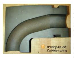
Carbinite is a carbide coating that is electrofused to a base metal to add texture. This texture increases the coefficient of friction between the clamping surface and workpiece the allowing for a strong, solid grip
