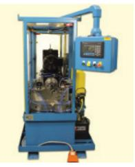
The 24014 high pressure/high thrust groover
