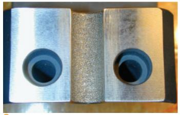
Clamp die with Carbinite coating
