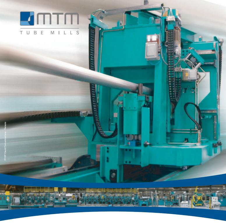
MTM Comby A200 series orbital flying cut off machines
