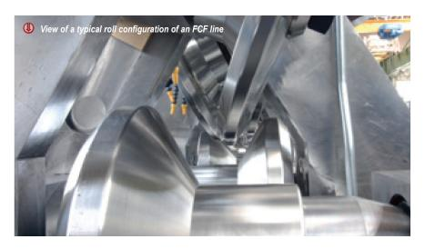
two inclined top rolls, universally applicable for several product dimensions. Welding in the FCF line is performed centrally along the mill centreline. Following welding of the profiles, final calibration of the square and rectangular sections is carried out in the FCF sizing section. The same set of universal tool rolls is used for the calibration of the final section dimensions and corner radii as well as for product-size changes.
