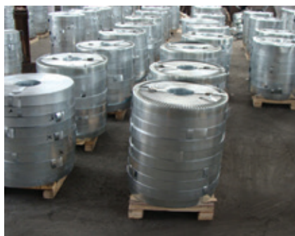
▲ Range of thicknesses for armouring cable strip
