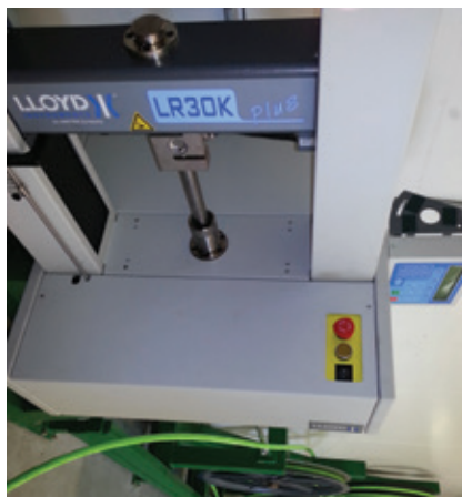
▲ 'Pogo' arrangement for LR30KPlus twin column materials testing instrument
