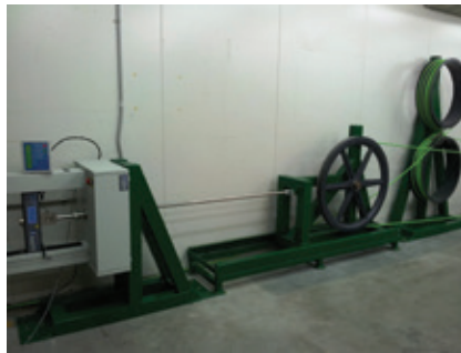
▲ Tensile testing assembly for optical fibres
