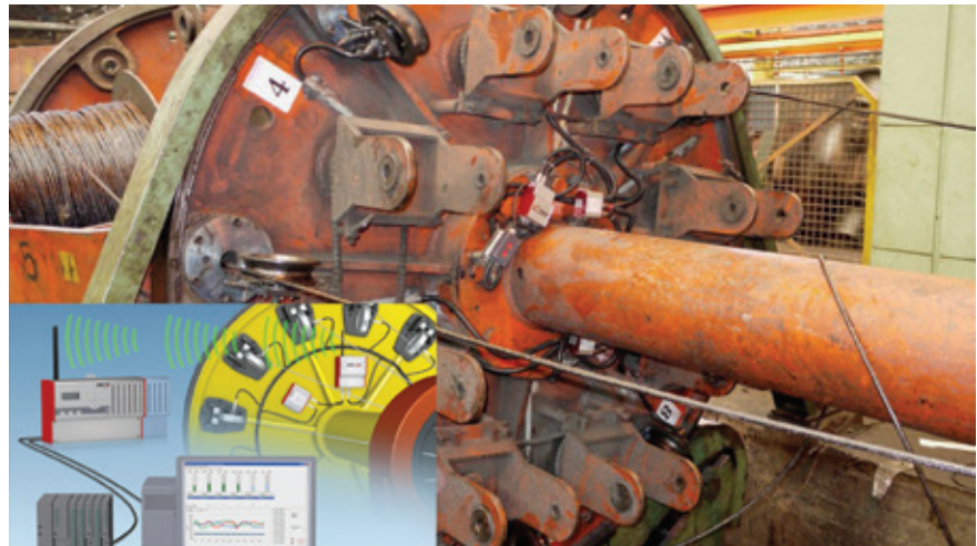
▲ A multi-stage planetary strander that was upgraded with FMS tension monitoring system RTMX42
