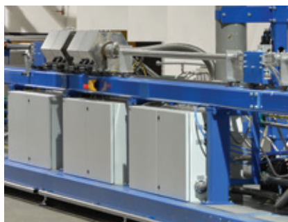
▲ PlasmaAnnealer for high speed annealing of fine SS wire
