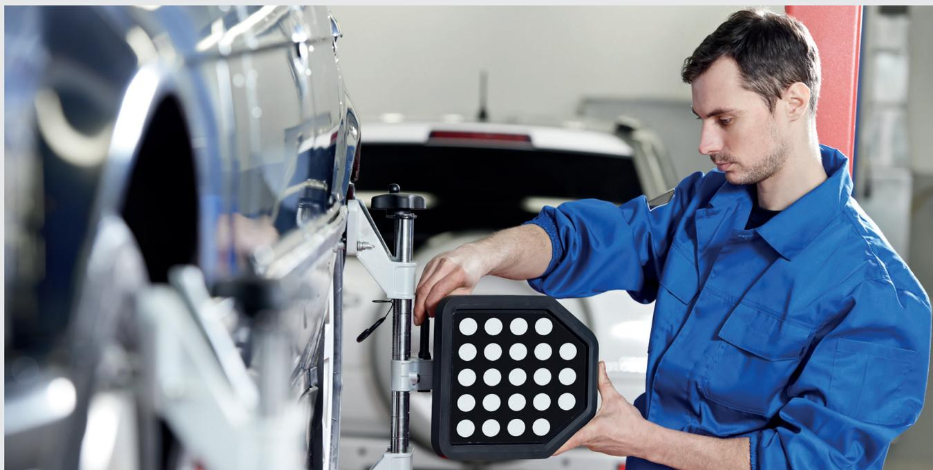
Every vehicle that comes into the workshop is an opportunity for a wheel alignment check, age, mileage and general wear and tear on **steering components, bearings** and **control arms** either wear out or fall out of adjustment, as well as, more commonly hitting a pothole or banging into a curb can often throw a vehicle out of alignment.
