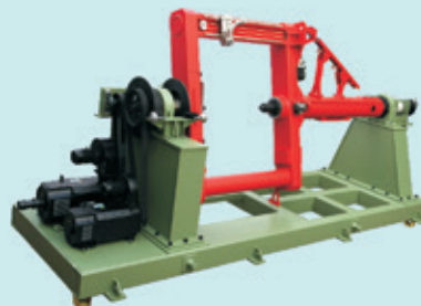
DJΦ1250-2000 Single twisting machine with armoring
