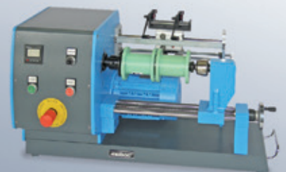
Spooler for spools Ø 60 - 200 mm, available with one or two spool seats, with revolution counter to preset and automatic stop, with spool take up via adjustable pintle and follower tip available with mechanical or laser sensor controlled traverse unit
