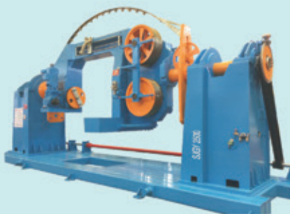
SJΦ1000-Φ2500 Double twist stranding machine
