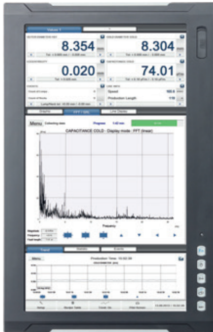
▲ At the vertical, 22" wide-screen monitor of the Ecocontrol 6000, FFT analysis and production data are clearly displayed
