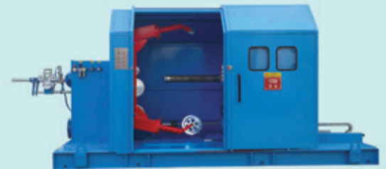
XBΦ500-Φ2500 Cantilever type single twisting machine
