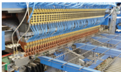
▲ FSD fence line welding portal
