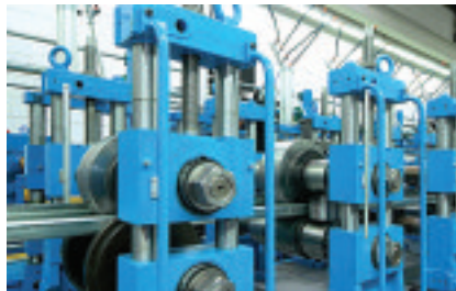
ⓘ The P3.200 rollforming machine is used to manufacture profile cross sections
