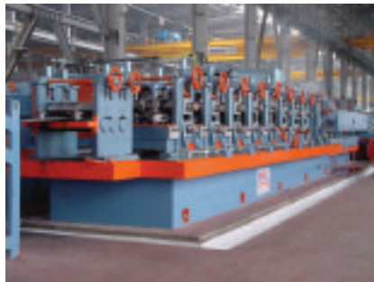
A tube mill for the production of welded tube
