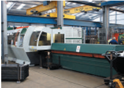
i The Adige LT712D LaserTube installed in IAE's new 65,000ft 2 manufacturing facility can cut and profile tube up to 152mm diameter
