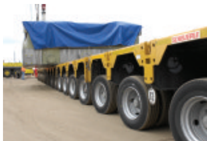
ⓘ Fully loaded, the special transporter truck had a weight of 355 tons
