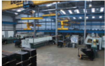
i IAE's new BLM TS72 CNC saw sits between the LT712D LaserTube (right) and the smaller LT652 tube laser
