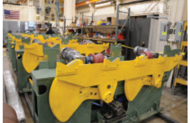
ⓘ A Bronx rotary straightener, recently delivered and installed
