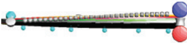
Picture 12: The standard design of roll tooling with Copra (tube mill module, cage design functions) with constant centre of gravity
