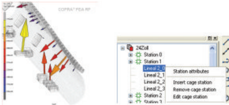
Picture 9: A feature of Copra is the possibility to design and model any type of rolling cage – often referred to as straight edge forming method. Using this feature, respective rolls are not just modeled but also transferred to Copra’s integrated finite element software package Copra® FEA RF and simulated respectively
