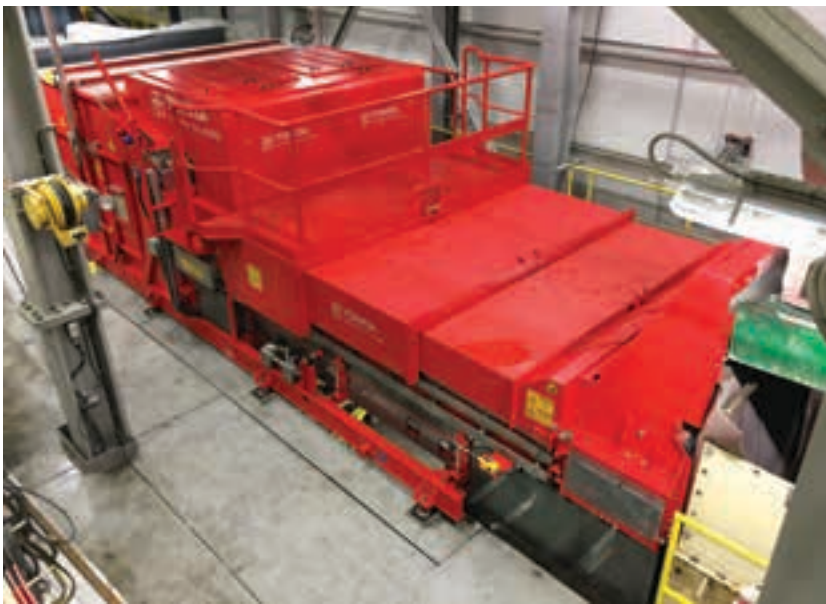
The Renard mine of Stornaway in Quebec, Canada, is the first diamond mine in the world with LDR in its primary flowsheet (photo: Stornaway).
