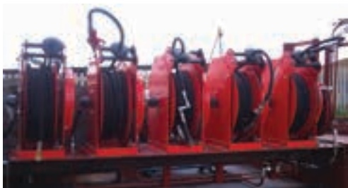
Pumprite heavy duty retractable reels are used for high performance transfer of lubricants and abrasive fluids.
