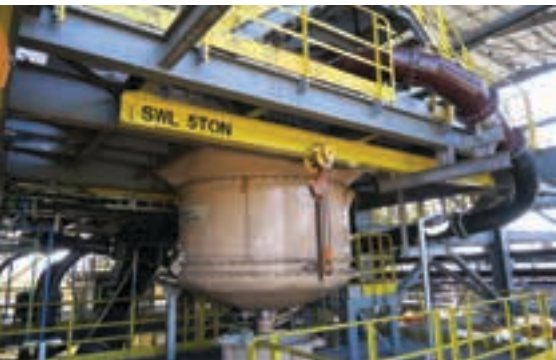
This photo illustrates the underflow arrangement of a REFLUX™ Classifier.
