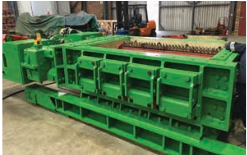
A Series 625 secondary sizer (segment machine) ready for delivery to West Africa.
