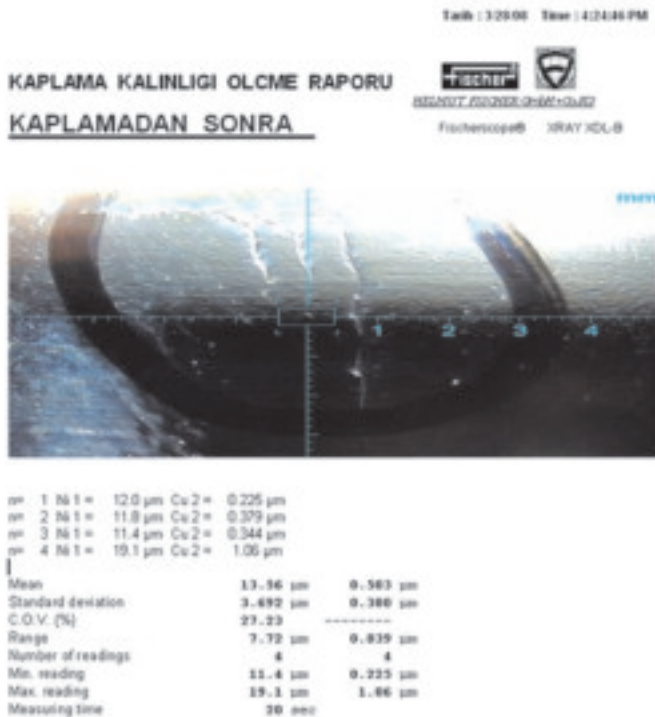
Figure 2: Scratches that do not disappear after electroplating
