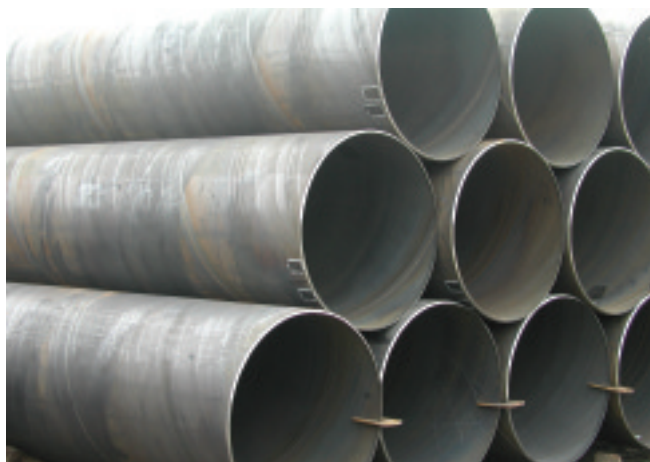
US Steel Košice produces spiral-welded pipes up to 1,422mm
