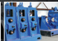
16" Cage Forming HF Tube Mill Line
