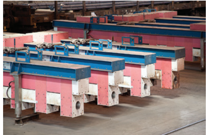
Easy change-over of the induction coils to a different diameter
