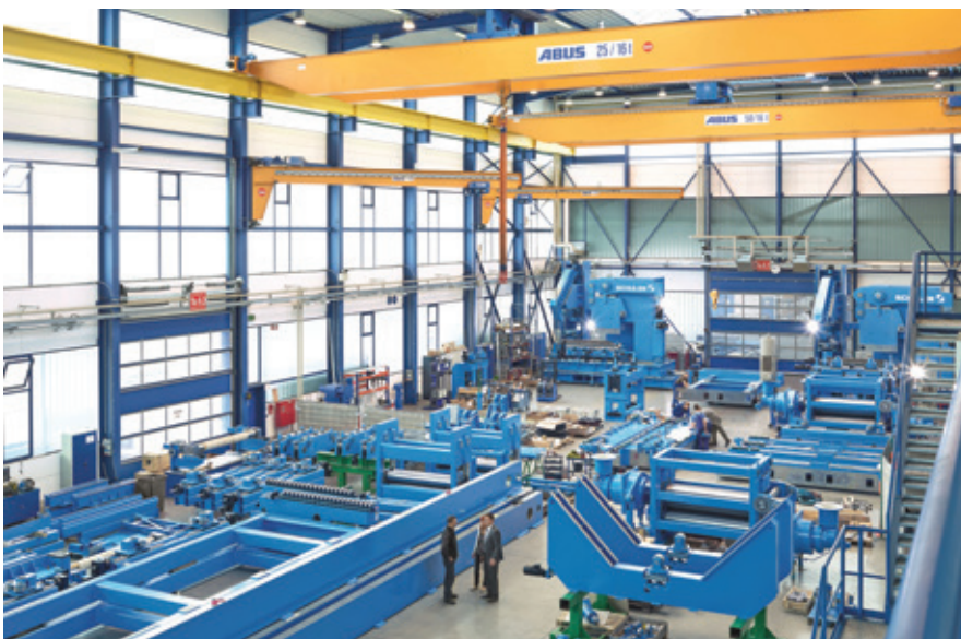
Pre-assembly of the two spiral pipe mills has been completed
