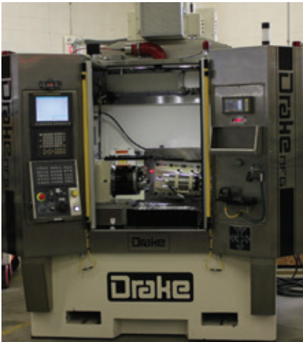
Drake GS:TI internal thread grinder for conventional EPS ball nuts
