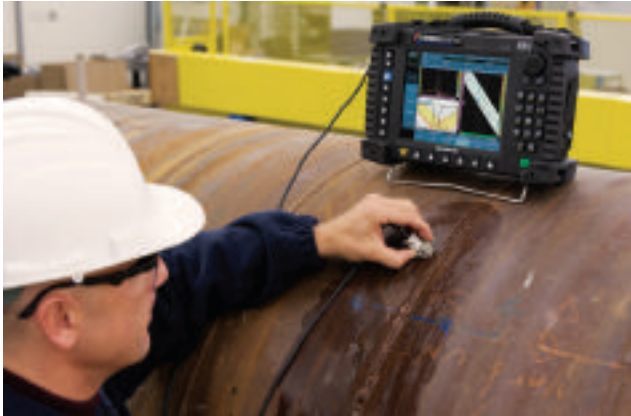
▲ The portable OmniScan features a large colour display that can be read under any lighting conditions
