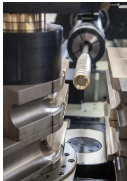
Due to the eight-stack tooling, set-up can be as simple as changing a mandrel
