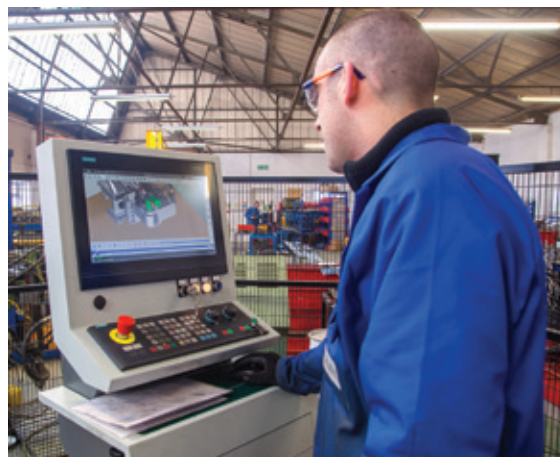
The control on the BLM Elect 102 stores operating parameters to simplify set-up
