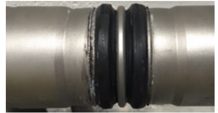
MetaPlex seal after completing V0 test cycle and recovered to smaller than its original diameter
