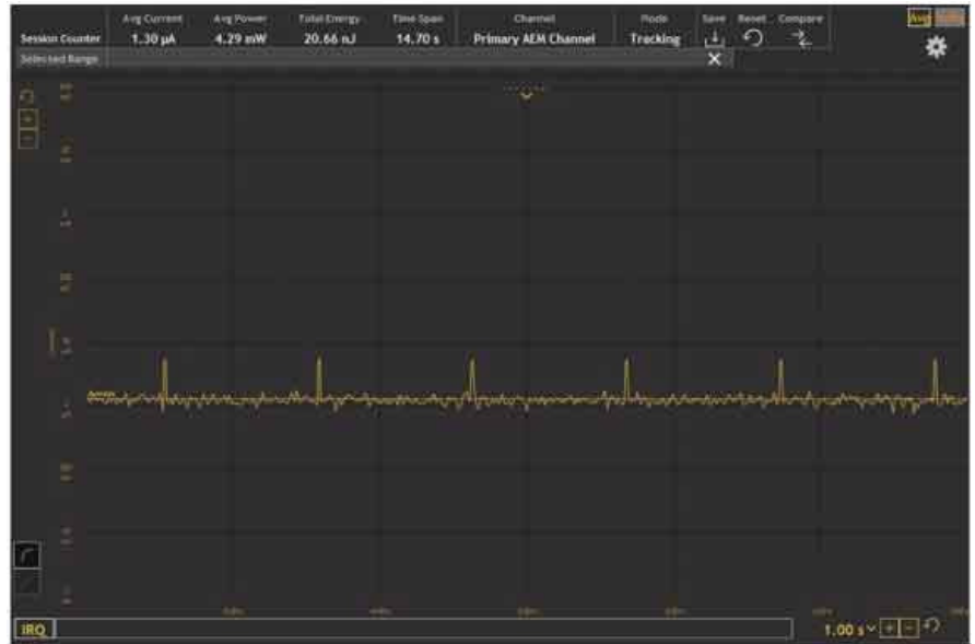
Figure 3 - Wonder Gecko, EM2 interrupt driven, sampling ADC @ 1 Hz.
