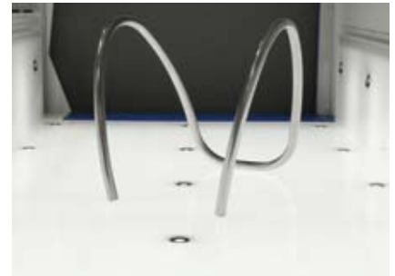
Free-form tube placed in the TubelInspect measuring cell
