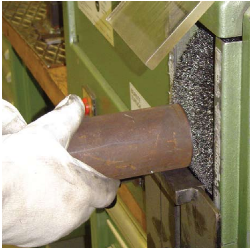
Manual de-burring of cut edges with brushes
