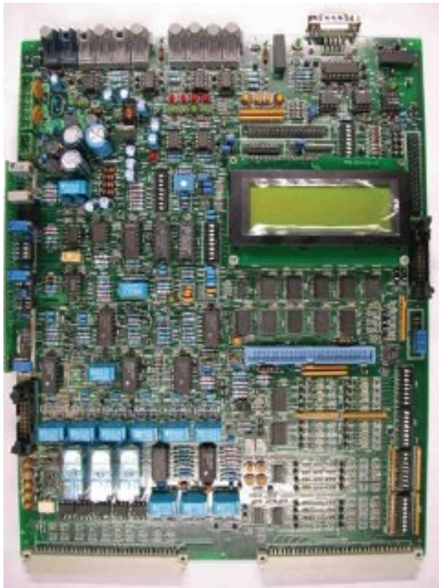
Figure 6: Digital supervising board
