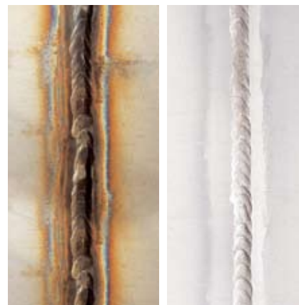
Before and after: weld of a stainless steel sheet, cleaned and passivated with Polinox-Protect to improve corrosion resistance
