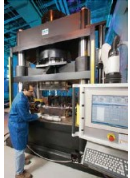
Interlaken's hydroforming technology
