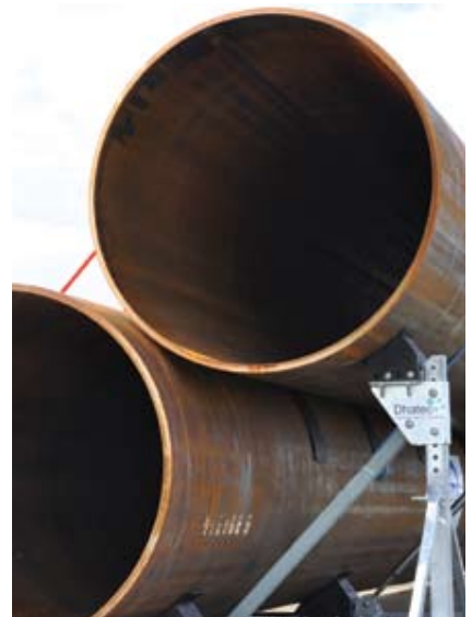
Dhatec's Pipe Raiser system places one pipe above another, to reduce the width of the total load
