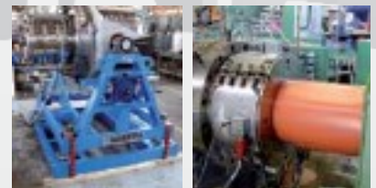
Newly designed dies for HDPE and PVC (also Foam layers) pipes
