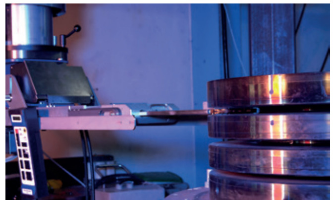
Figure 11: Turbine rotor welding module
