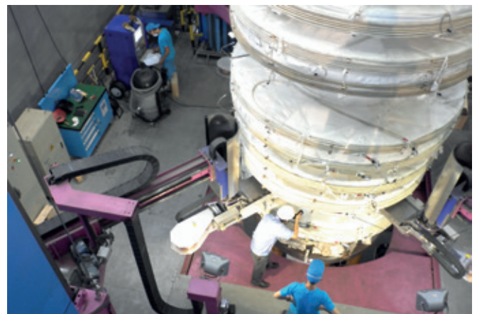
Figure 2: Turbine rotor welding with thicknesses of up to 300–400mm
