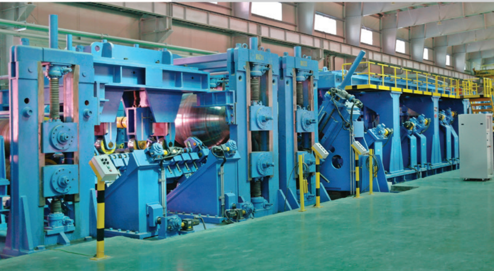
CAGE FORMING SECTION / PIPE MILL 8" -24"Ø
