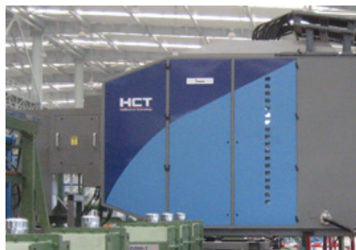
Patented Thermatool® HAZControl™ technology 800kW dual welder
