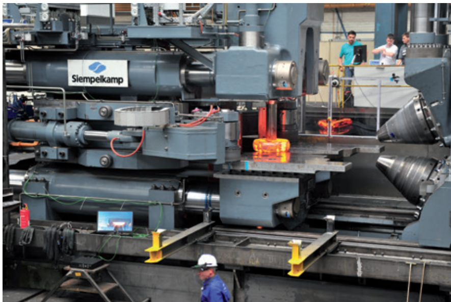
The rings are made of billets manufactured on another Siempelkamp press
