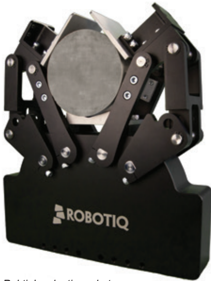
Robotiq's adaptive robot gripper in encompassing grip mode
