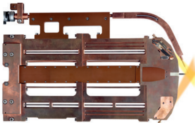
Figure 6: NG torch with integrated front and rear cameras
