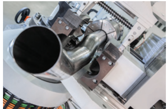
The transfluid machine permits bending radii of 1 x D and more for tubes with diameters up to 127mm while reducing wall thicknesses from 2 to 1.5mm
