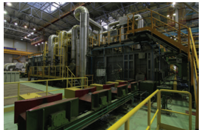
The walking beam furnace, which will be similar to the one shown above, will be equipped with SMS Prometheus software to achieve improved heat efficiency
