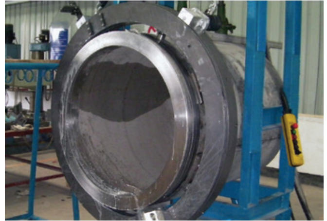
Figure 11: Protem clamshell TTNG1016. 32"-40" heavy wall thickness – Material: austenitic stainless steel
