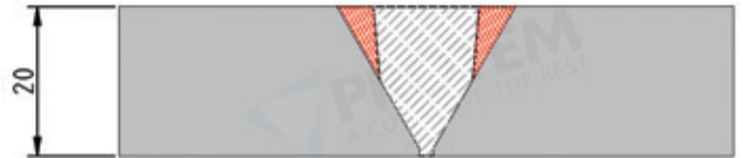
Figure 4: Material saving for a compound bevel on a wall thickness of 20mm
