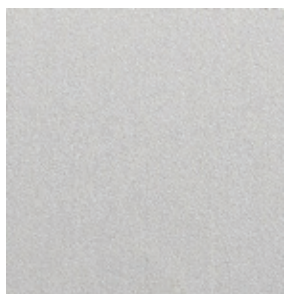
Figure 1: Finishing obtained through the “HFree” process – alloy UNS S32750
