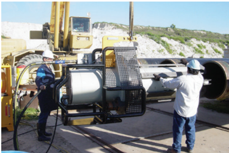
Figure 8: Application example: Producing a bevel at the end of a pipe, on-site, for an onshore pipeline
